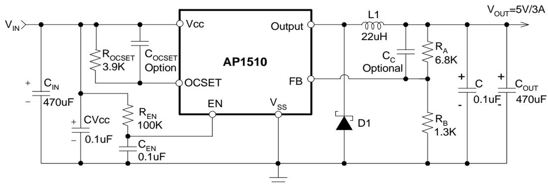
Note:  $V_{OUT} = V_{FB} \times (1 + R_A/R_B)$
