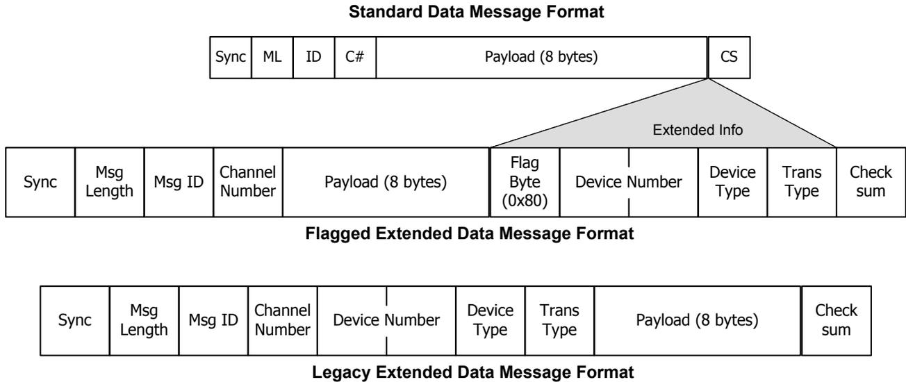
**Figure 7-2. Extended Data Messages, Flagged and Legacy Formats.**
