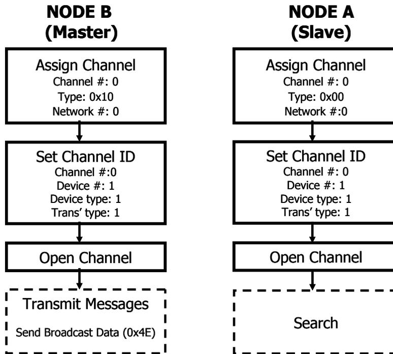
Figure 8-2. Node A & B Channel Establishment
