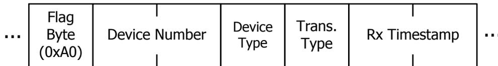
**Figure 7-6. Channel ID and Rx timestamp enabled**
