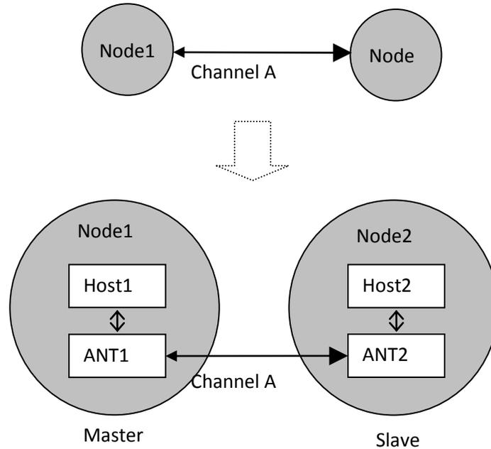
**Figure 5-1. Channel communication between two ANT nodes**
