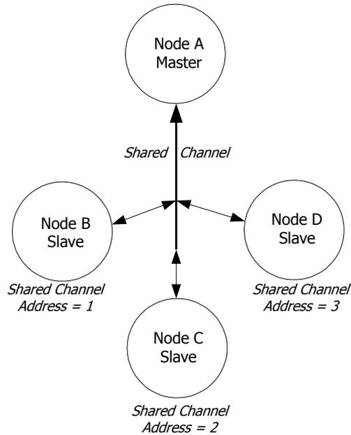
**Figure 8-4. Shared channel implementation of sample network**
