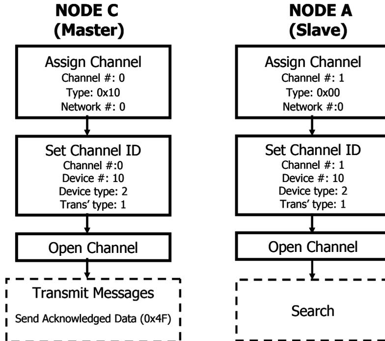
Figure 8-3. Node C & A Channel Establishment
