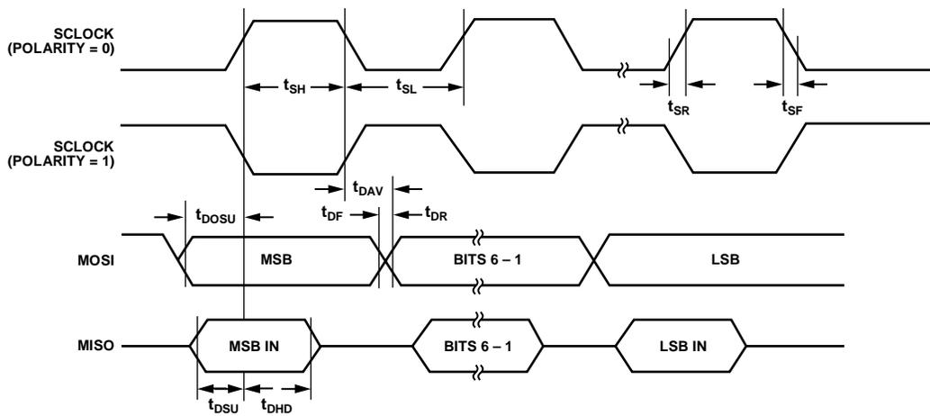
Figure 3. SPI Master Mode Timing (PHASE Mode = 0)
