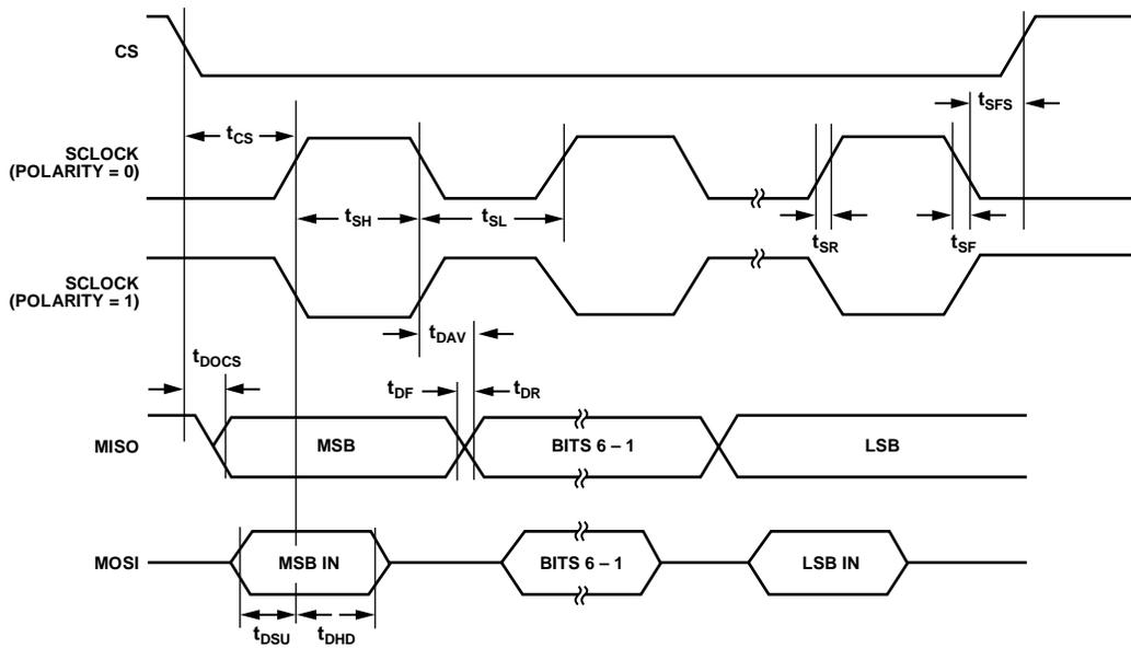
Figure 5. SPI Slave Mode Timing (PHASE Mode = 0)
