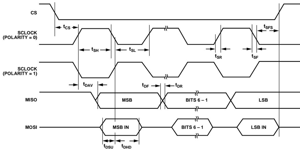
Figure 4. SPI Slave Mode Timing (PHASE Mode = 1)
