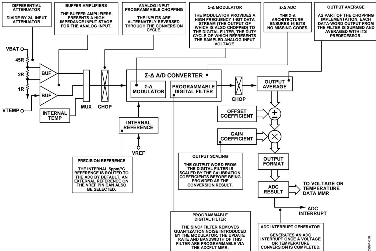
Figure 16. Voltage/ Temperature ADC, Top Level Overview
