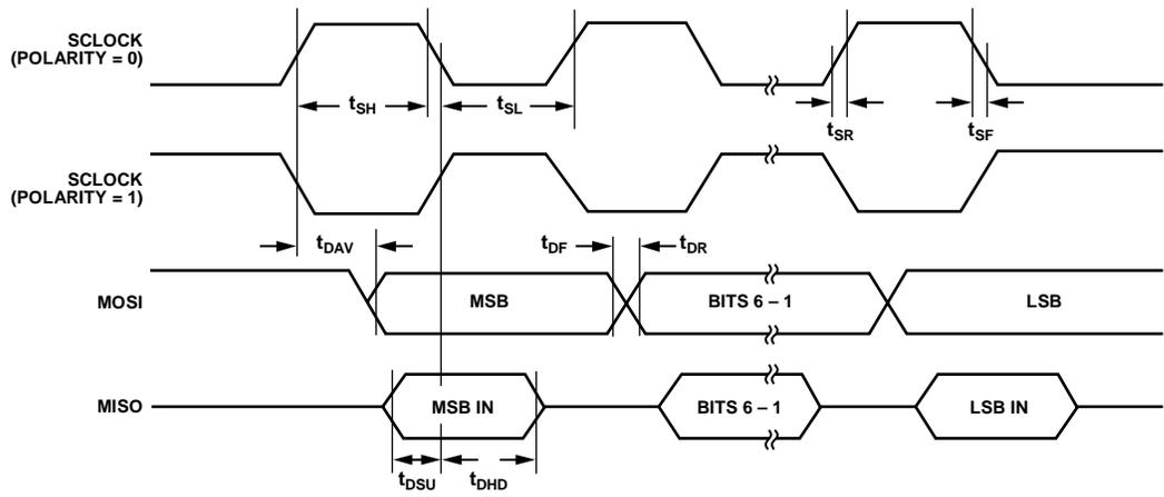
Figure 2. SPI Master Mode Timing (PHASE Mode = 1)
