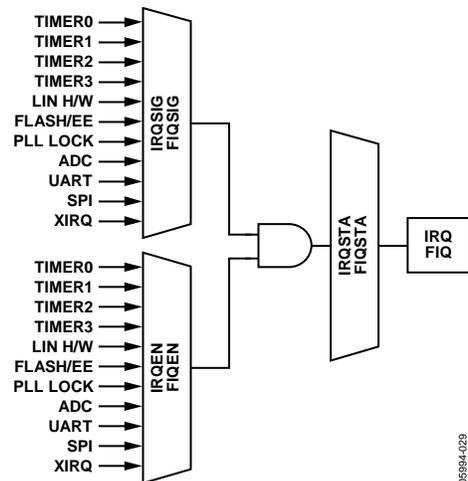
Figure 29. Interrupt Structure
