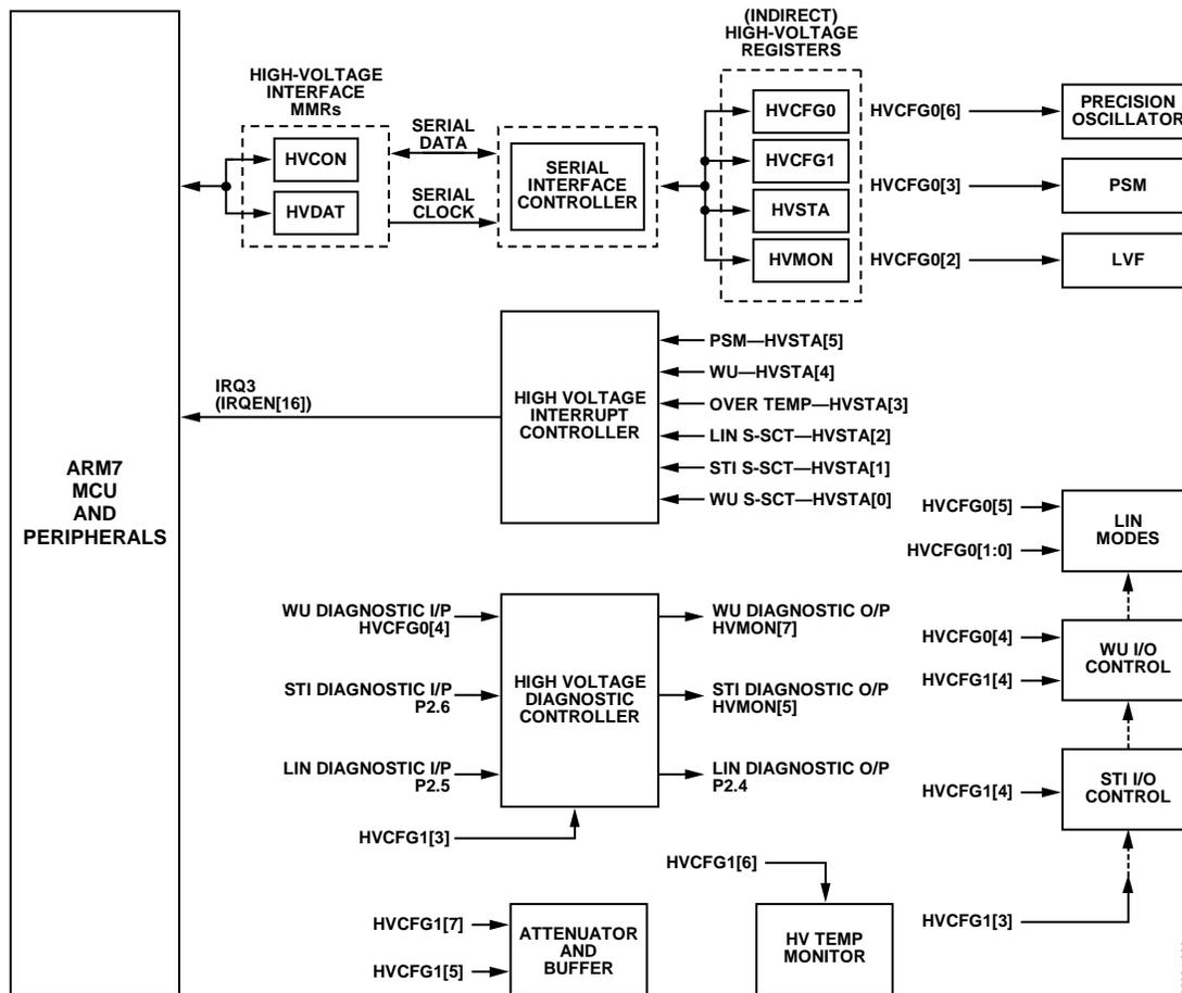
Figure 36. High Voltage Interface, Top Level Block Diagram
