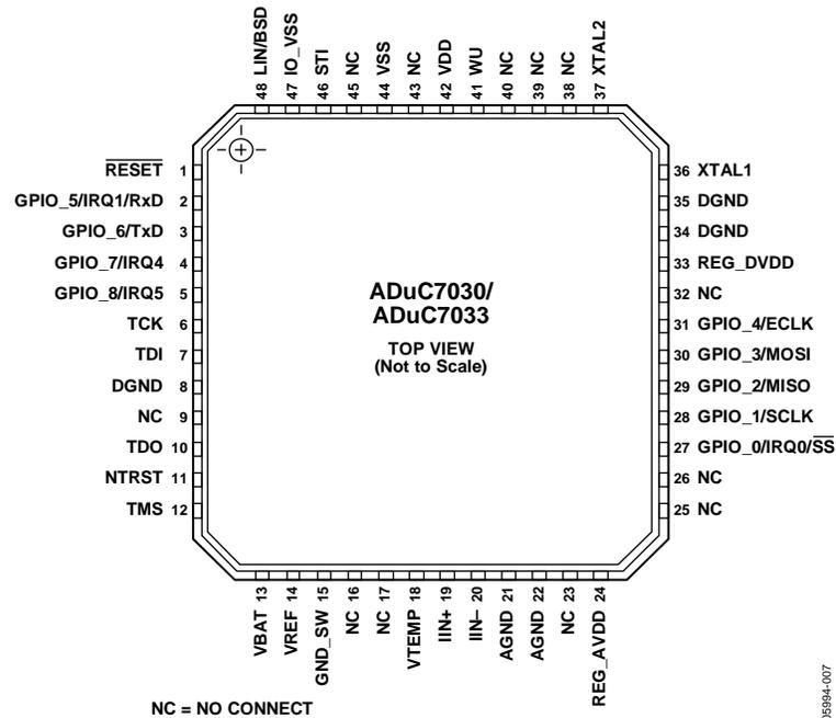
Figure 7. Pin Configuration
