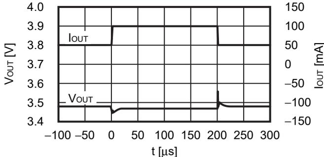
3. Transient response characteristics of ON / OFF pin ( $T_a = +25^\circ\text{C}$ )
