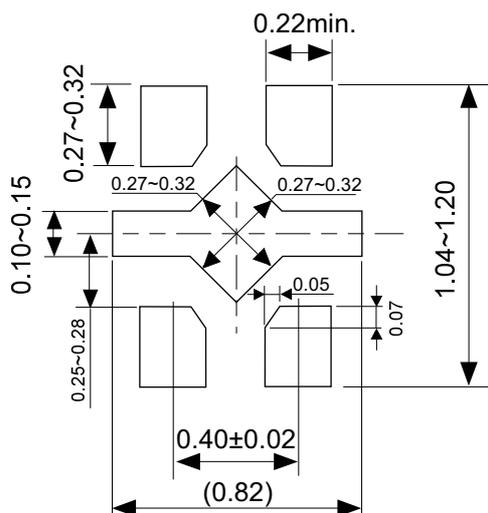
Caution It is recommended to solder the heat sink to a board in order to ensure the heat radiation.
