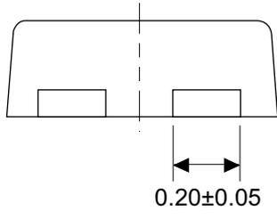
※ The heat sink of back side has different electric potential depending on the product. Confirm specifications of each product. Do not use it as the function of electrode.
