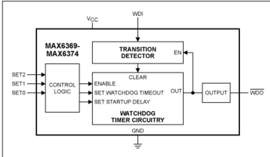
Figure 8. Block diagram of Maxim's pin-selectable watchdog-timer ICs.
