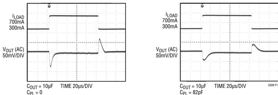
**Figure 11. Transient Load Response with Different Combinations of  $C_{OUT}$  and  $C_{PL}$  Load Current Step from 300mA to 700mA**
