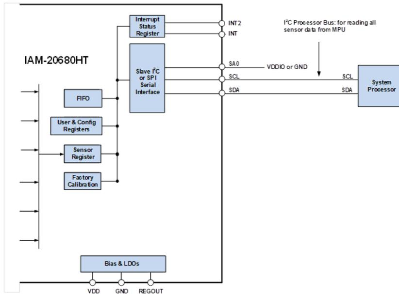
Figure 6. IAM-20680HT Solution Using I<sup>2</sup>C Interface
