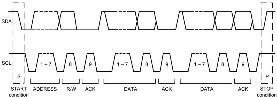
**Figure 10. Complete I<sup>2</sup>C Data Transfer**
