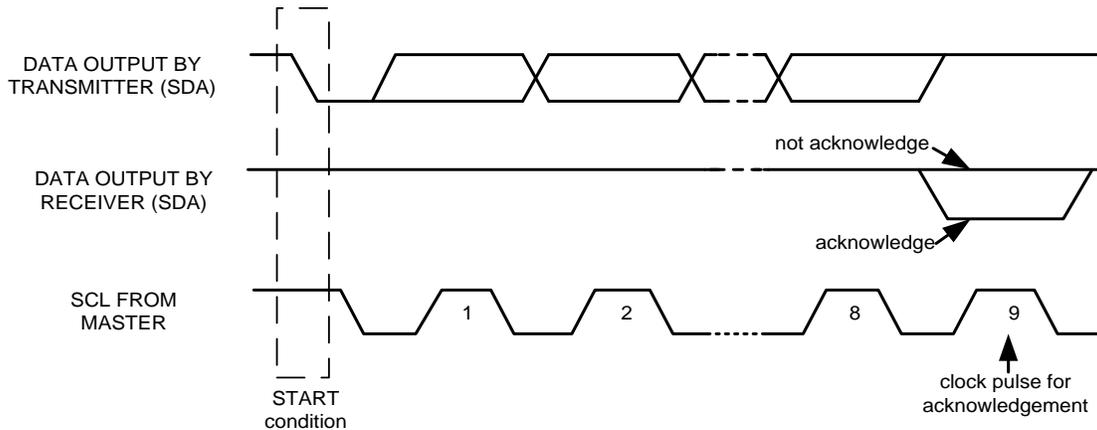
**Figure 9. Acknowledge on the I<sup>2</sup>C Bus**
