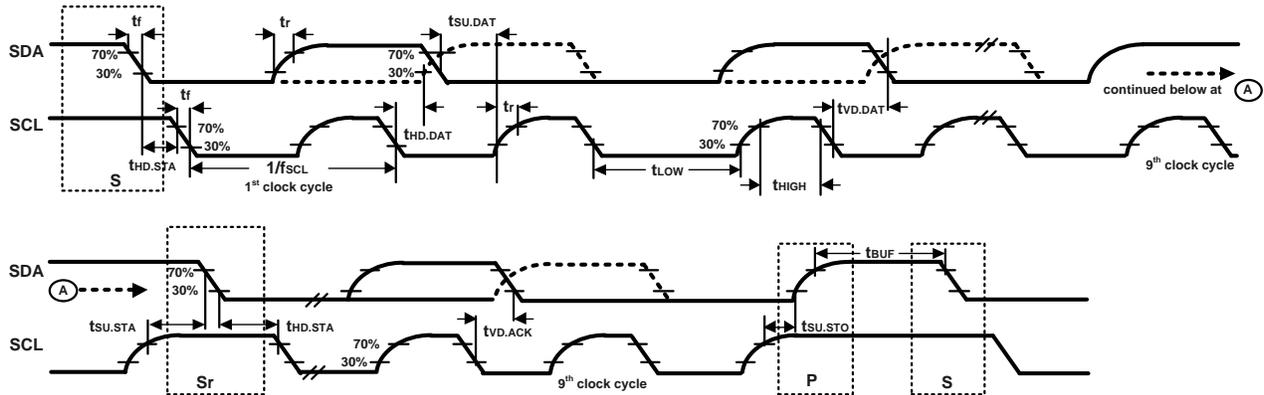
Figure 1. I<sup>2</sup>C Bus Timing Diagram
