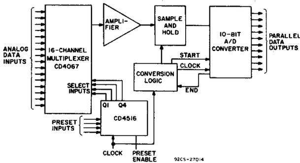
This acquisition system can be operated in the random access mode by jamming in the channel number at the preset inputs, or in the sequential mode by clocking the CD4516B.
