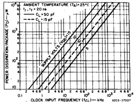
Fig. 9 - Typical dynamic power dissipation vs. frequency.
