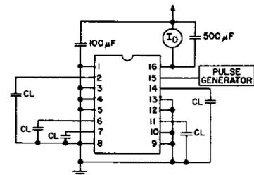
Fig. 14 - Power-dissipation test circuit and input waveform.
