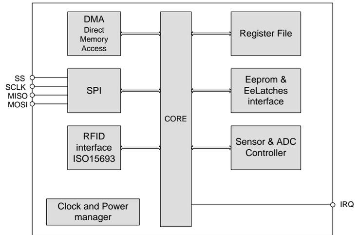
The digital controller manages the transactions between the communication interfaces, the memories and the sensor. It allows also a standalone mode with its DMA unit. All these blocks are described in the next chapters.
