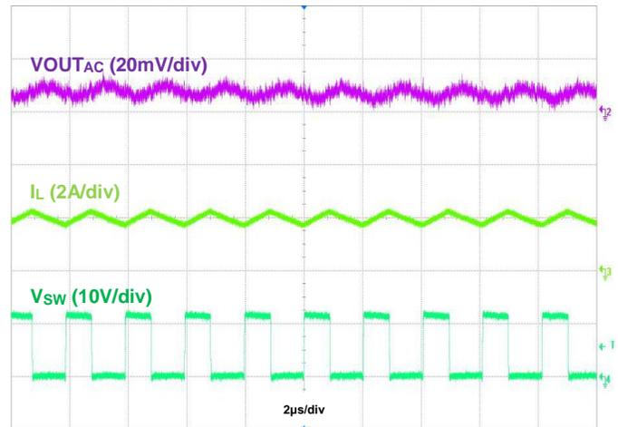
Figure 15. Output Voltage Ripple,  $V_{OUT} = 5\text{V}$ ,  $I_{OUT} = 2\text{A}$
