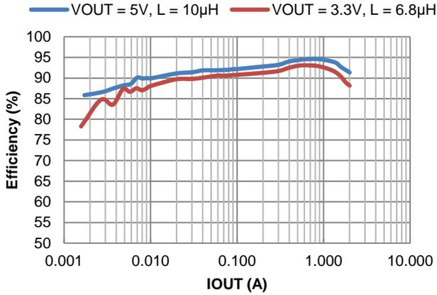
Figure 4. Efficiency vs. Output Current,  $V_{IN} = 12\text{V}$
