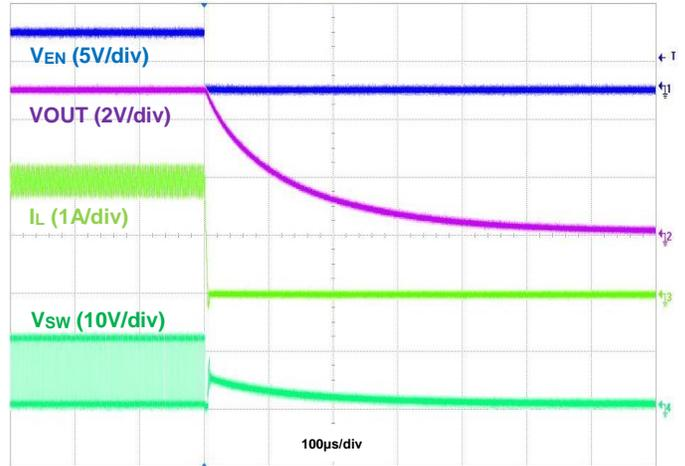
Figure 22. Shutdown Using EN, IOU = 2A
