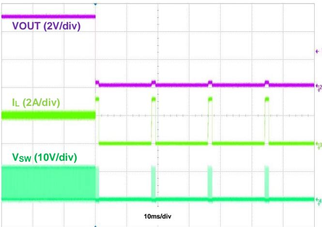
Figure 23. Output Short Protection, IOU = 2A
