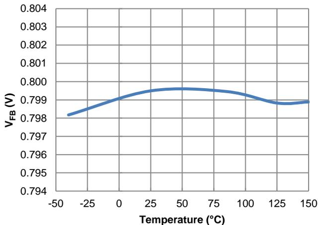
Figure 8. Feedback Voltage vs. Temperature,  $I_{OUT} = 1\text{A}$
