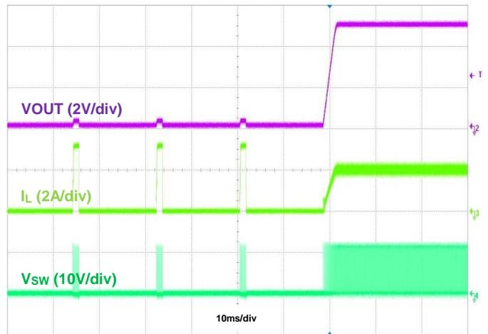
Figure 24. Output Short Recovery, IOU = 2A
