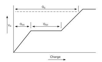
Basic gate charge waveform
