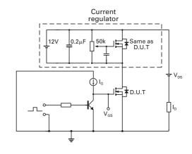
Gate charge test circuit
