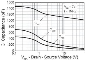
Capacitance v Drain-Source Voltage
