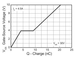
**Gate-Source Voltage v Gate Charge**
