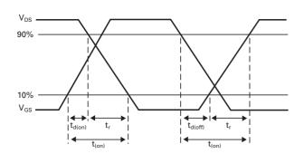
Switching time waveforms
