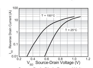
Source-Drain Diode Forward Voltage
