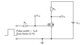
Switching time test circuit
