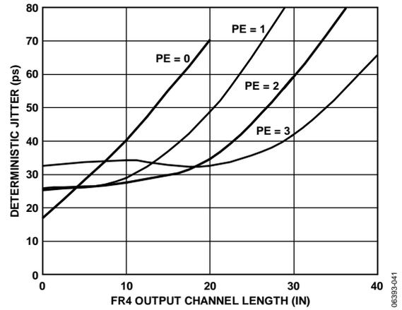
Figure 20. Deterministic Jitter vs. FR4 Output Channel Length
