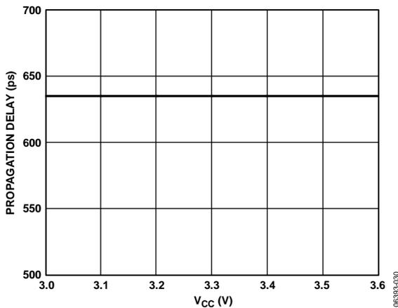
Figure 25. Propagation Delay vs. Core Supply Voltage
