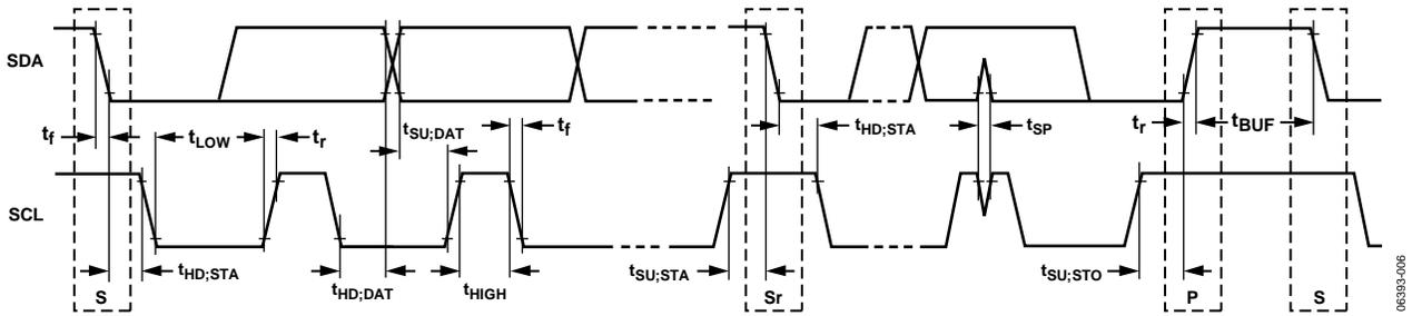
Figure 2. I<sup>2</sup>C Timing Diagram
