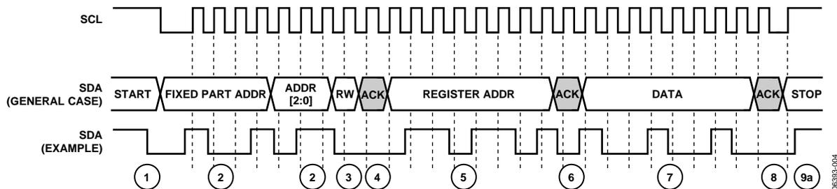
Figure 32. I<sup>2</sup>C Write Diagram
