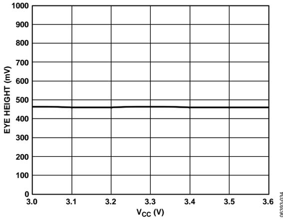
Figure 29. Eye Height vs. Core Supply Voltage
