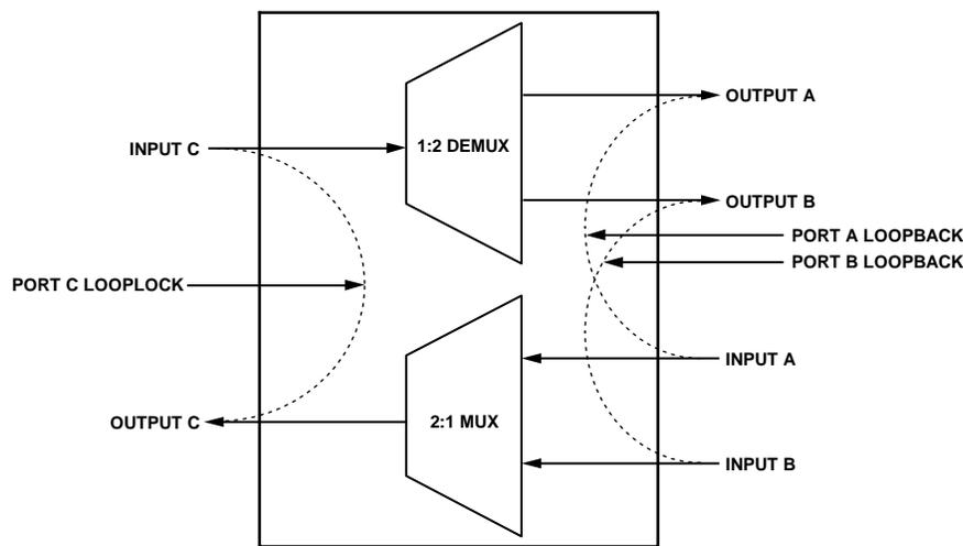
Figure 31. Loopback Configurations
