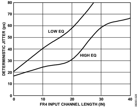
Figure 17. Deterministic Jitter vs. FR4 Input Channel Length
