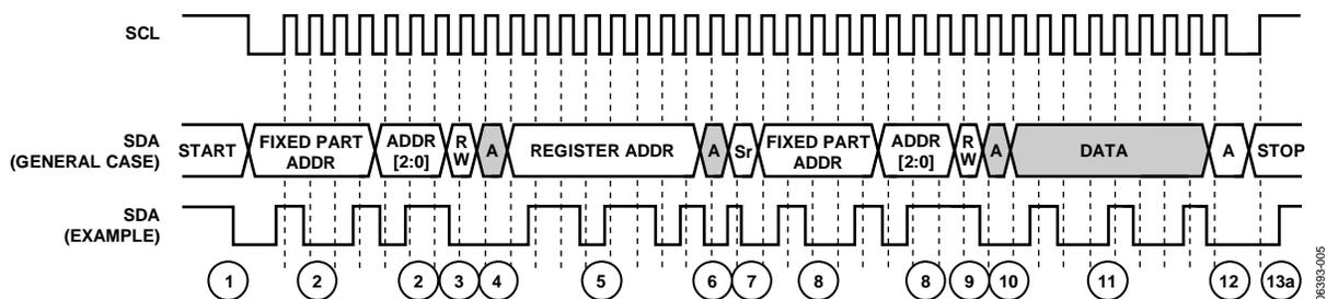
Figure 33. I<sup>2</sup>C Read Diagram
