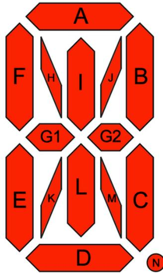
The bitmask is a 16-bit number that can be passed in as a single Hexidecimal, Decimal, or binary number. It can also be passed in as a list or tuple containing 2 separate 8-bit numbers. Here are some of the ways to set the digits. All of these different methods create a box with an X in the center:
