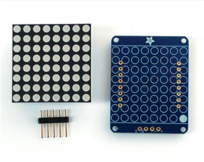
When you buy a pack from Adafruit, it comes with the fully tested and assembled backpack as well as a 8x8 matrix in one of the colors we provide (say, red, yellow or green). You'll need to solder the matrix onto the backpack but it's an easy task.
