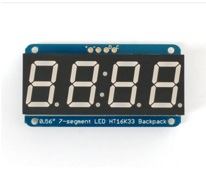
Remove the parts from packaging and place the LED matrix OVER the silkscreen side. **DO NOT PUT THE DISPLAY ON UPSIDE DOWN OR IT WONT WORK!!** Check the image below to make sure the 'decimal point' dots are on the bottom, matching the silkscreen.
