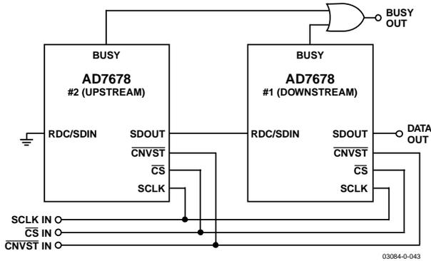
Figure 37. Two AD7678s in a Daisy-Chain Configuration
