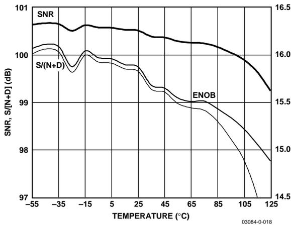
Figure 13. SNR, S/(N+D), and ENOB vs. Temperature
