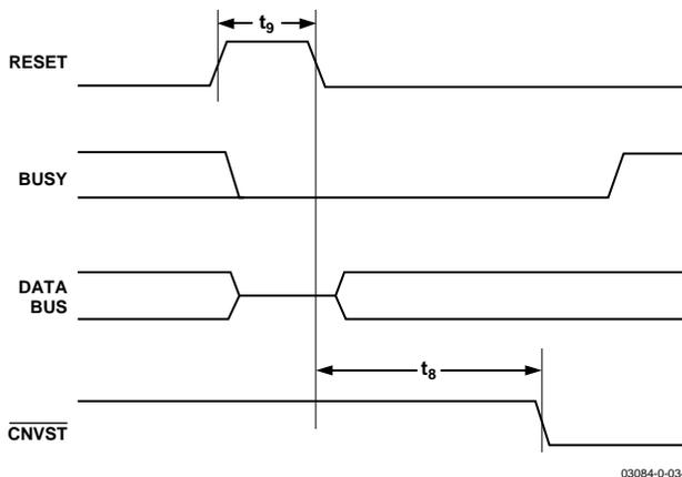
Figure 28. RESET Timing
