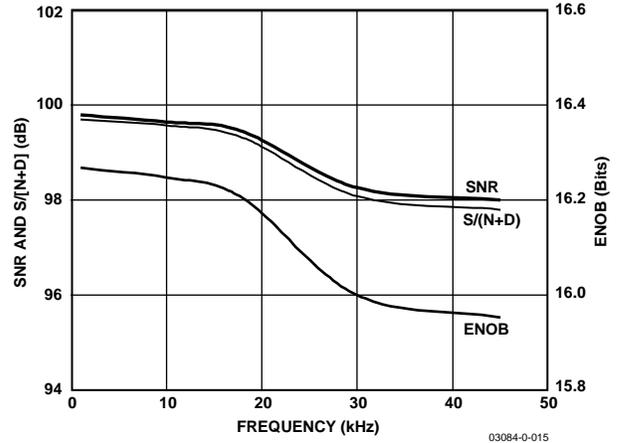
Figure 10. SNR, S/(N+D), and ENOB vs. Frequency
