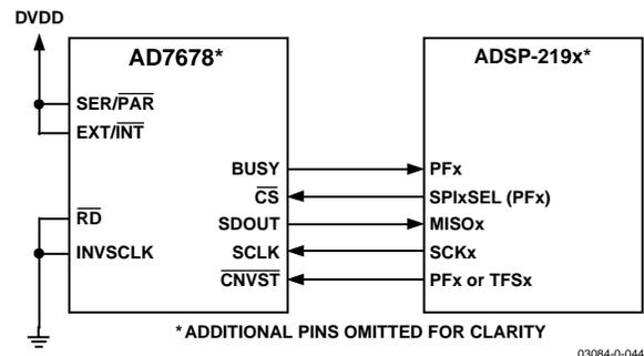
Figure 38. Interfacing the AD7678 to an SPI Interface
