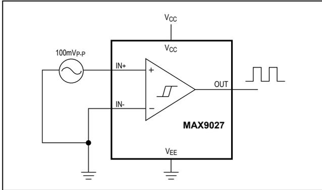
Figure 4. Zero-Crossing Detector
