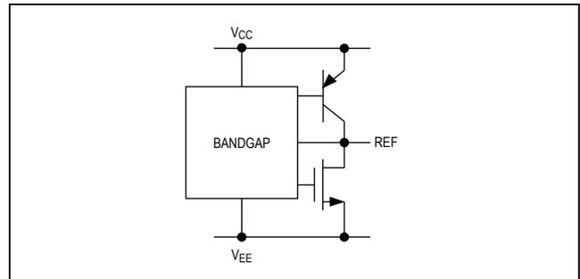
Figure 1. MAX9025/MAX9026 Voltage Reference Output Equivalent Circuit
