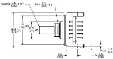
$$\begin{split} & \text{DIMENSIONS: } \frac{\text{MM}}{\text{(IN)}} \\ & \text{TOLERANCES: EXCEPT WHERE NOTED} \\ & \text{DECIMALS: .XX} \pm \frac{.51}{(.020)}.\text{XXX} \pm \frac{.13}{(.005)} \end{split}$$
