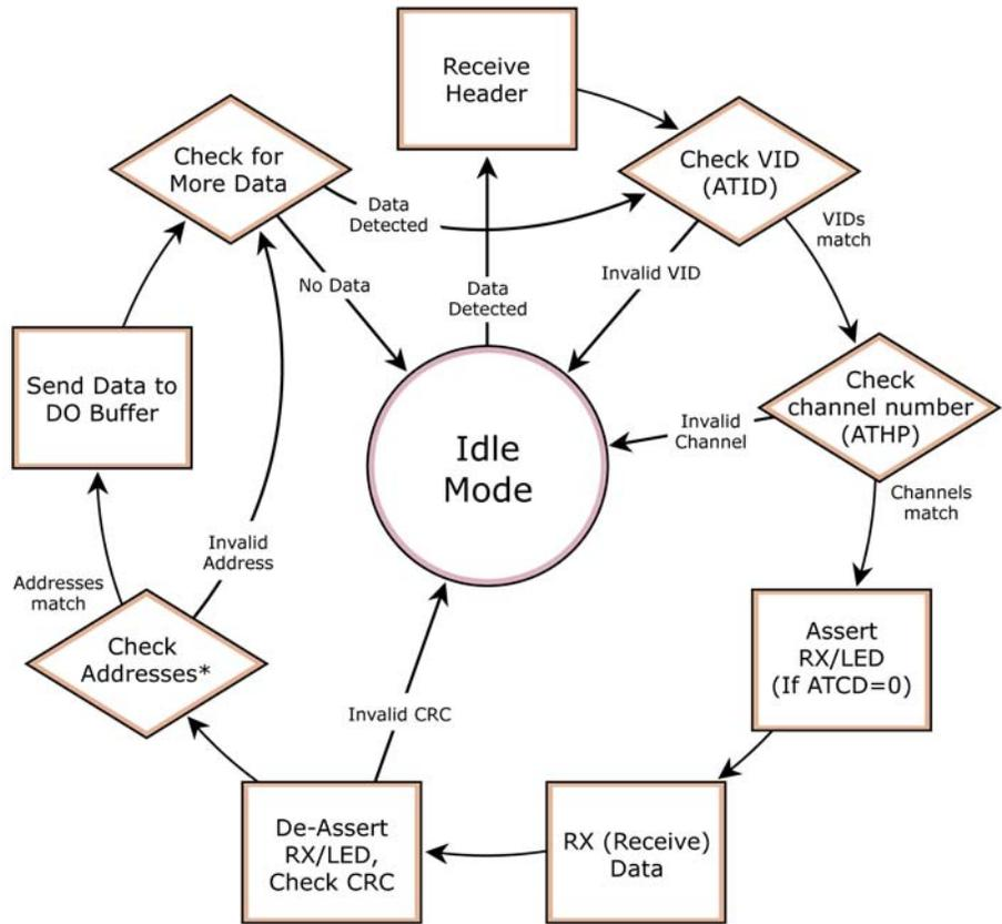
The modem returns to Idle Mode after valid data is no longer detected or once an error is detected in the received data. If serial data-to-transmit is stored in the DI buffer while the modem is giving precedence to Receive Mode, the data will be transmitted after the modem finishes receiving data and returns to Idle Mode.
