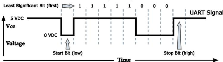
In the example above, the MaxStream RF modem transfer 8 bits over-the-air [Selectable using BI (Number of Bits) Parameter]. Start and stop bits of the UART signal are not transmitted over-the-air, but are regenerated by the receiving modem
