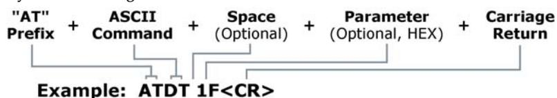
To read a parameter value stored in the modem register, leave the parameter field blank.
