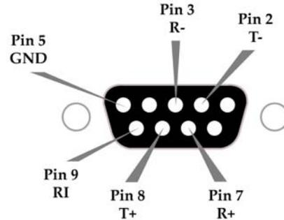
Table 2-03. RS-485/422 (4-wire) Signals and their implementations on the XCite RF Modem
