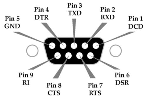
Table 2-01. RS-232 Signals and their implementations on the XCite RF Modem
