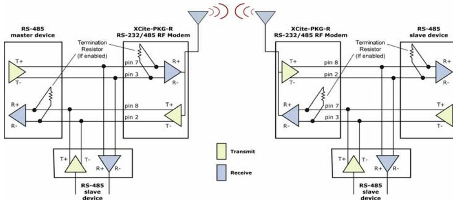
Figure 2-14. XCite RF Modem in an RS-422 environment
