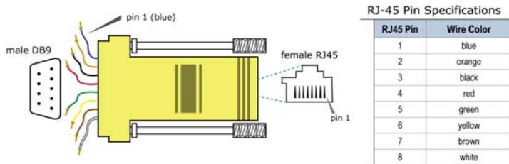
Figure 2-16. Female DB-9 to RJ-45 Adapter (green)
