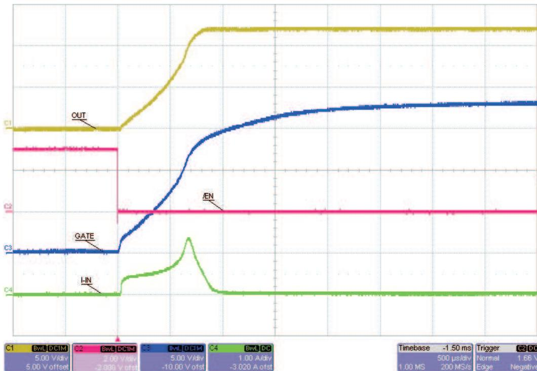
Figure 7. Typical Power Limited Inrush Start Up (No C<sub>EXT</sub>)
