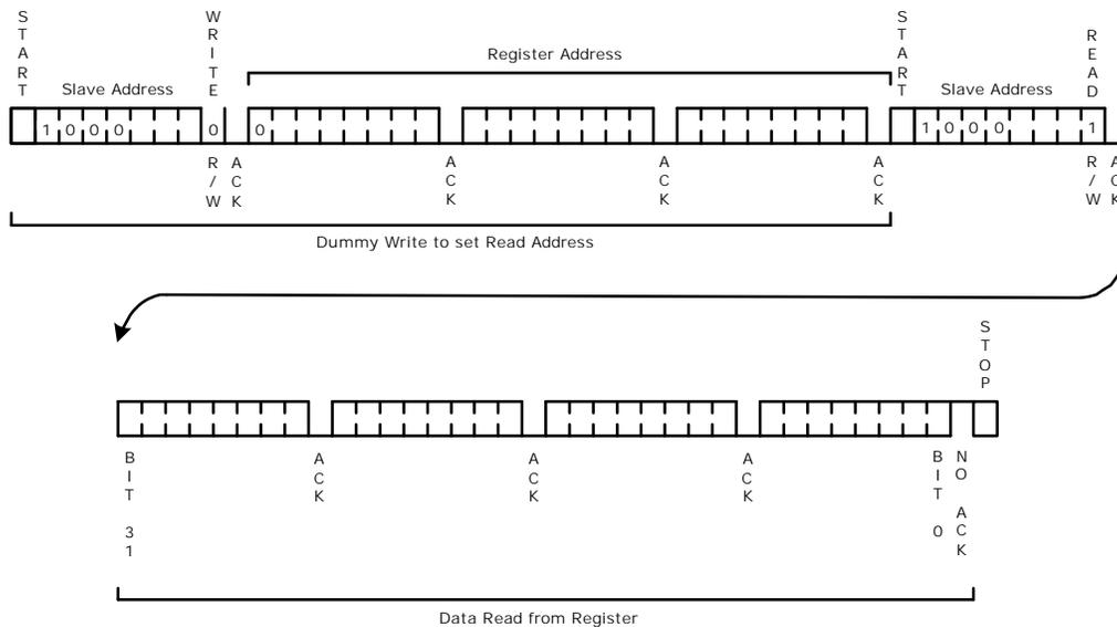
The two-wire serial slave interface supports sequential read and sequential write instructions.
