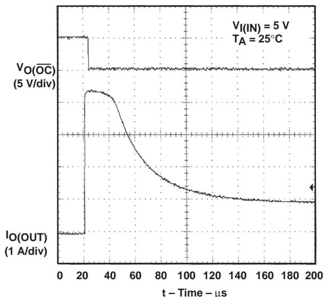
Figure 11. 1-Ω Load Connected to Enabled Device
