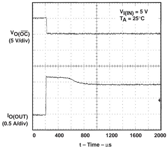
Figure 10. 4-Ω Load Connected to Enabled Device
