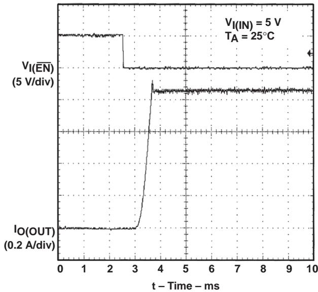
Figure 6. TPS2043, Short-Circuit Current, Device Enabled into Short
