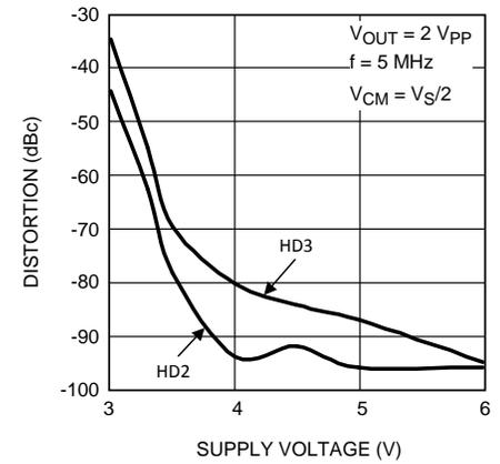
Figure 12. Distortion vs Supply Voltage (Split Supplies)
