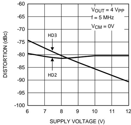
Figure 13. Distortion vs Supply Voltage (Single Supply)
