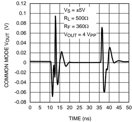
Figure 8. Output Common-Mode Pulse Response
