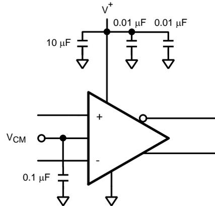
Figure 26. Single Supply Bypassing Capacitors
