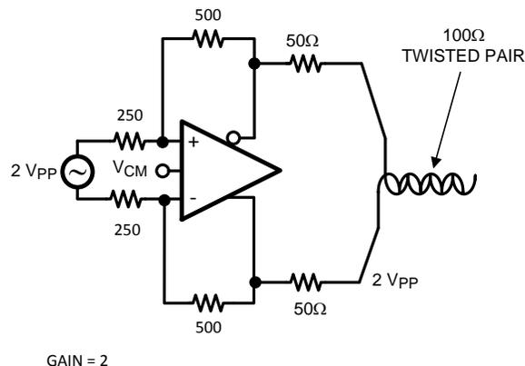
**Figure 24. Fully Differential Cable Driver**
