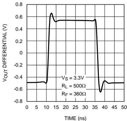
Figure 5. 1  $V_{PP}$  Pulse Response Single-Ended Input
