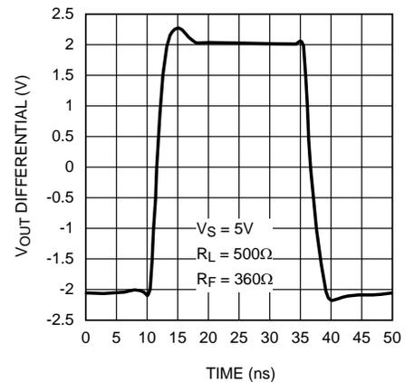
Figure 6. 2  $V_{PP}$  Pulse Response Single-Ended Input
