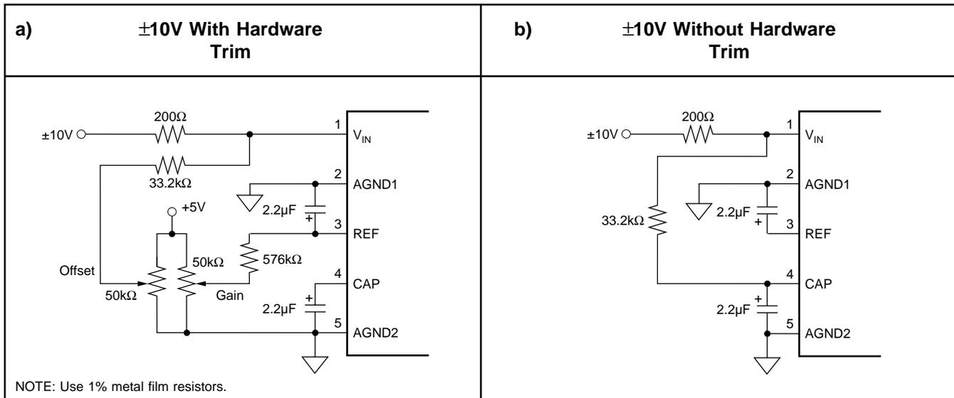
FIGURE 6. Circuit Diagram With and Without External Resistors.
