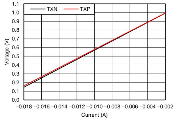
Figure 4-7. TX Termination I-V
