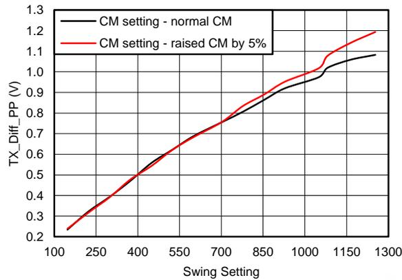
Figure 4-8. Diff TX Swing versus Swing Settings
