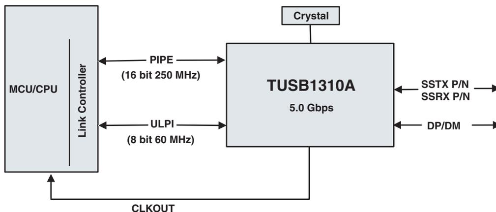
Figure 6-1. Typical Application Schematic
