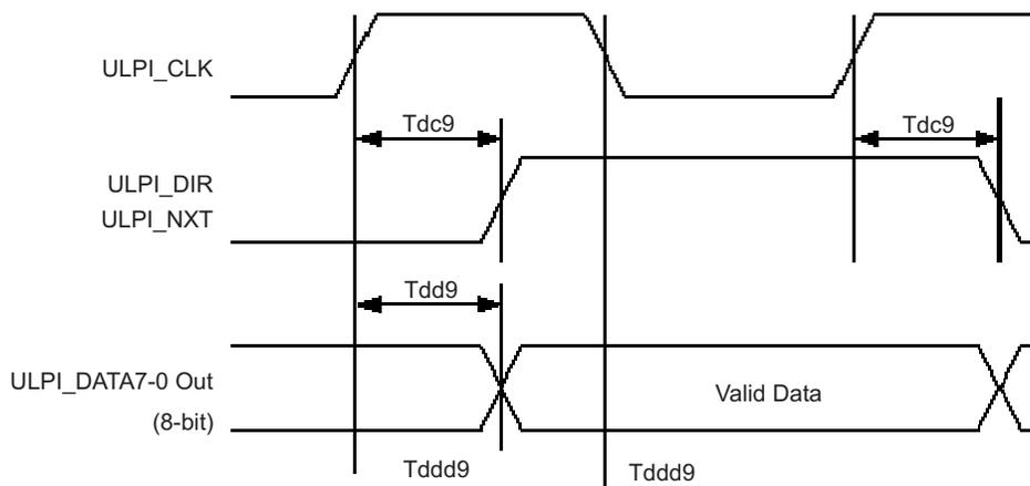
**Figure 4-5. ULPI Receive Timing**
