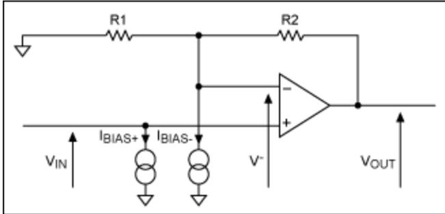
Figure 2. Current sources model input bias currents for the ideal op amp of Figure 1.
