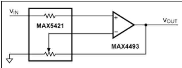
Figure 4. This precision amplifier combines precision resistors (MAX5421 ICs) with a general-purpose, rail-to-rail op amp (the MAX4493).
