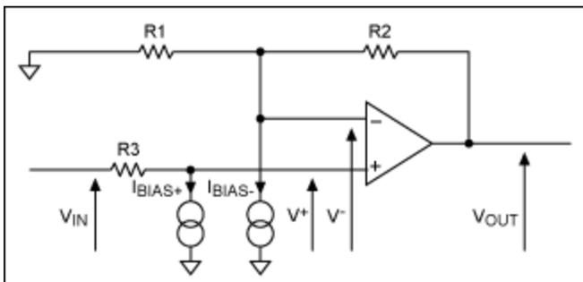
Figure 3. Adding a compensation resistor ( $R_3$ ) to the Figure 2 circuit cancels the effect of input bias currents.
