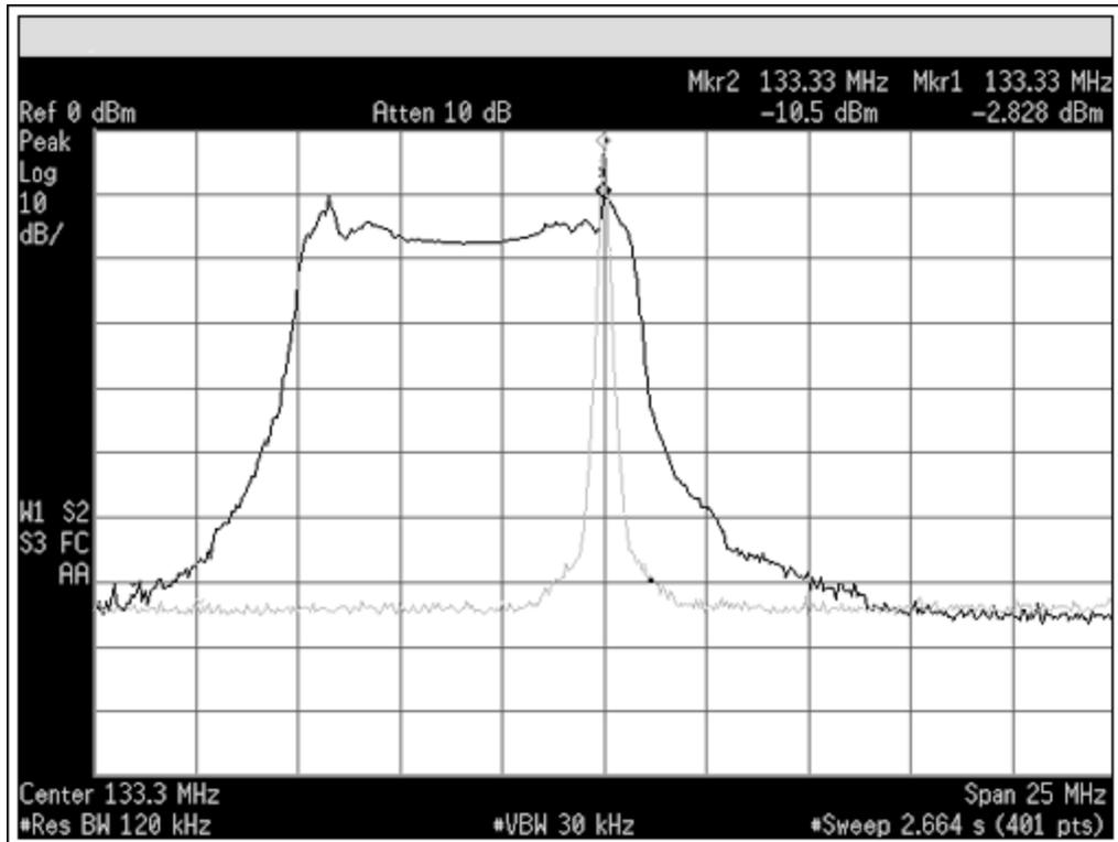
Figure 1. Clock spectrum of the DS4M133 with MS = low and MS = 8kHz (low to  $V_{CC}/2$ ) downspreading.
