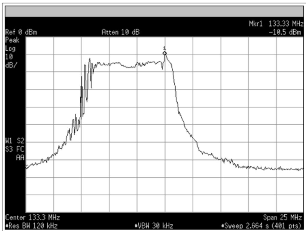
Figure 2. Clock spectrum of the DS4M133 with MS = 10kHz, low to V<sub>CC</sub>/2.
