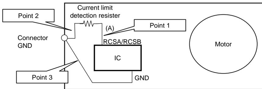
9) A high current flows into this LSI. Therefore, the common impedance of the PCB pattern cannot be ignored. Take the following points into consideration and design the PCB pattern of the motor.
