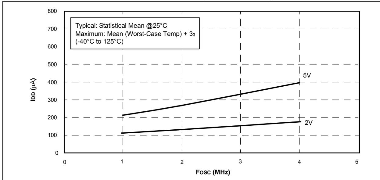
**FIGURE 12-2: MAXIMUM  $I_{DD}$  vs. Fosc OVER  $V_{DD}$  (XT, EXTRC mode)**
