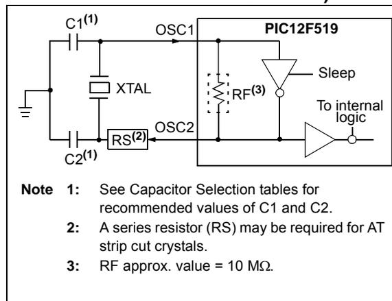
**FIGURE 8-2: EXTERNAL CLOCK INPUT OPERATION (XT OR LP OSC CONFIGURATION)**
