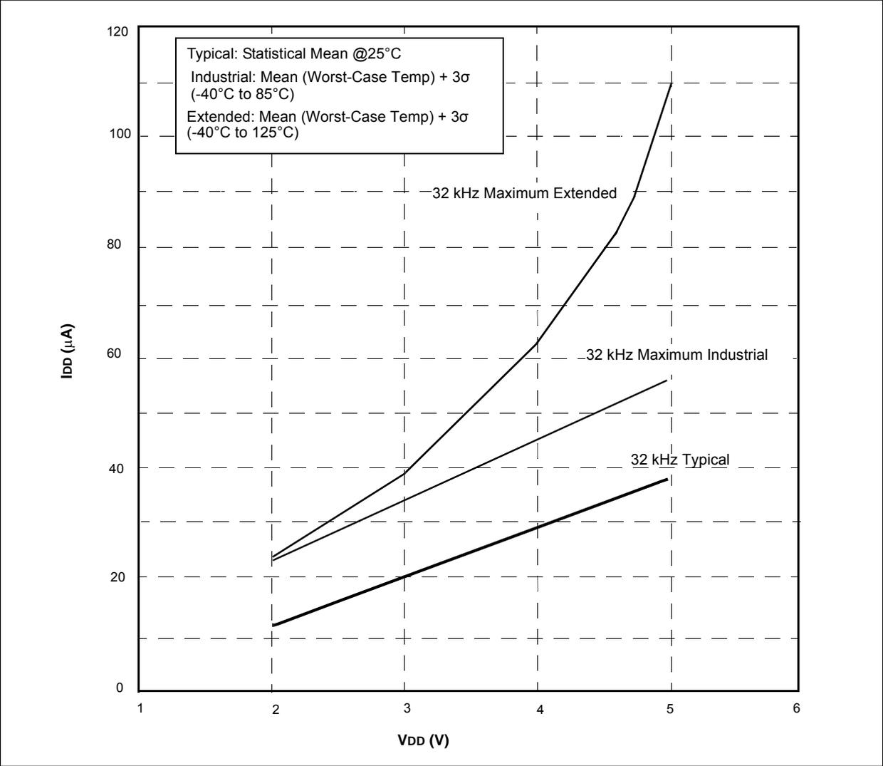
**FIGURE 12-4: TYPICAL IPD vs. VDD (SLEEP MODE, ALL PERIPHERALS DISABLED)**
