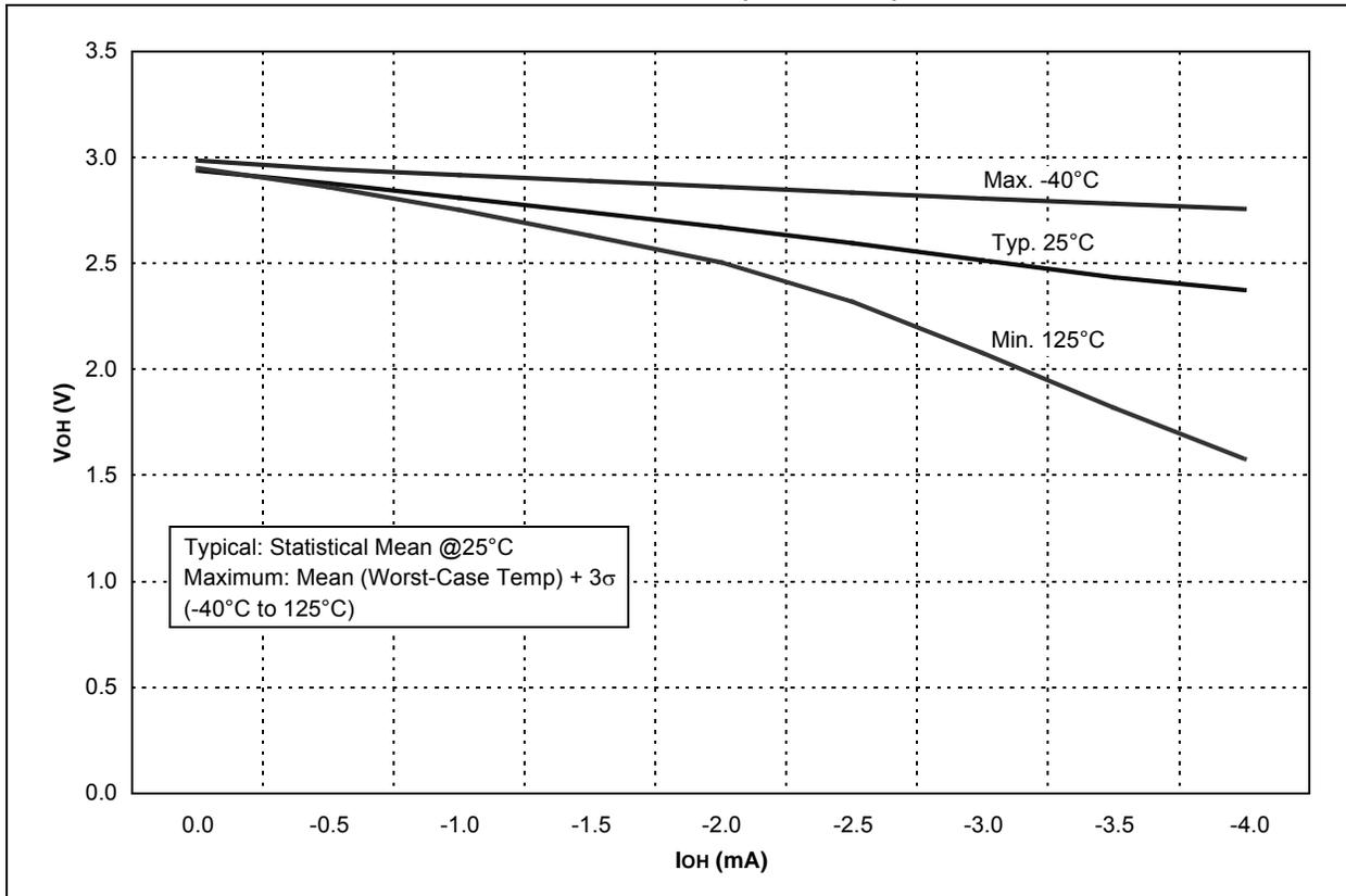
FIGURE 12-12:  $V_{OH}$  vs.  $I_{OH}$  OVER TEMPERATURE ( $V_{DD} = 5.0V$ )
