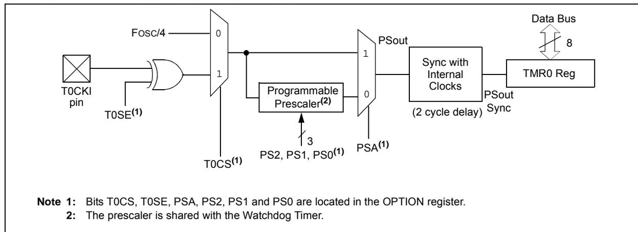
**FIGURE 7-2: TIMER0 TIMING: INTERNAL CLOCK/NO PRESCALE**
