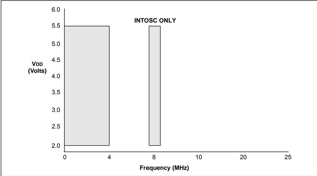
**FIGURE 11-2: MAXIMUM OSCILLATOR FREQUENCY TABLE**
