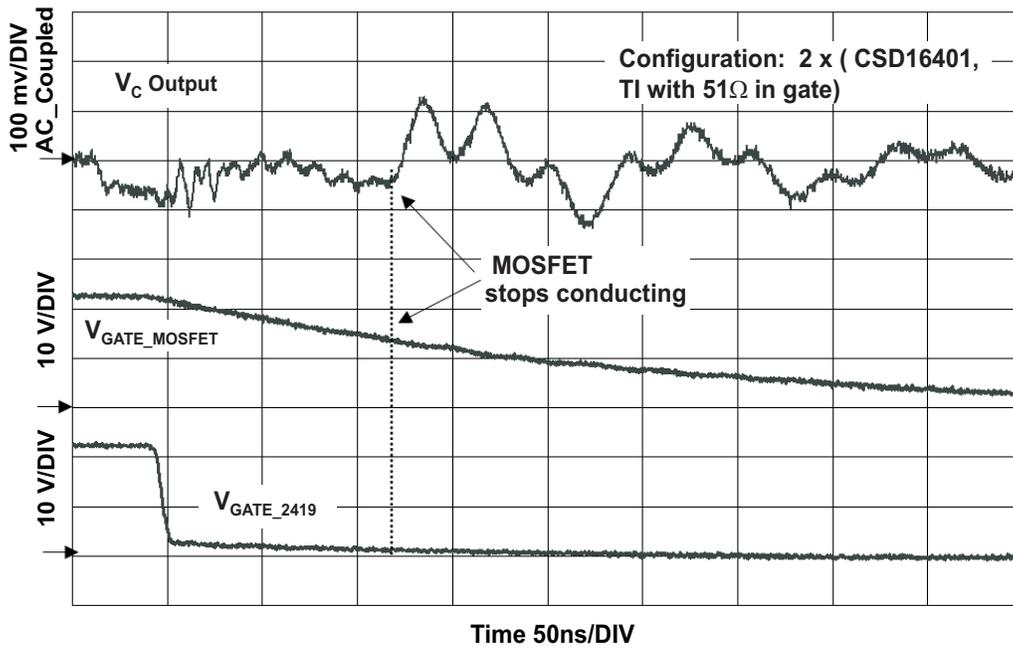
Figure 15. Gate Turnoff Waveforms with R<sub>GATE</sub> = 51Ω
