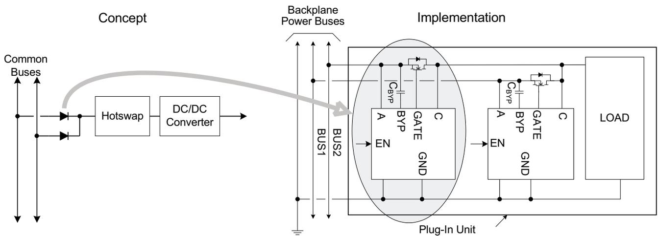
Figure 12. Example ORing of Input Power Buses
