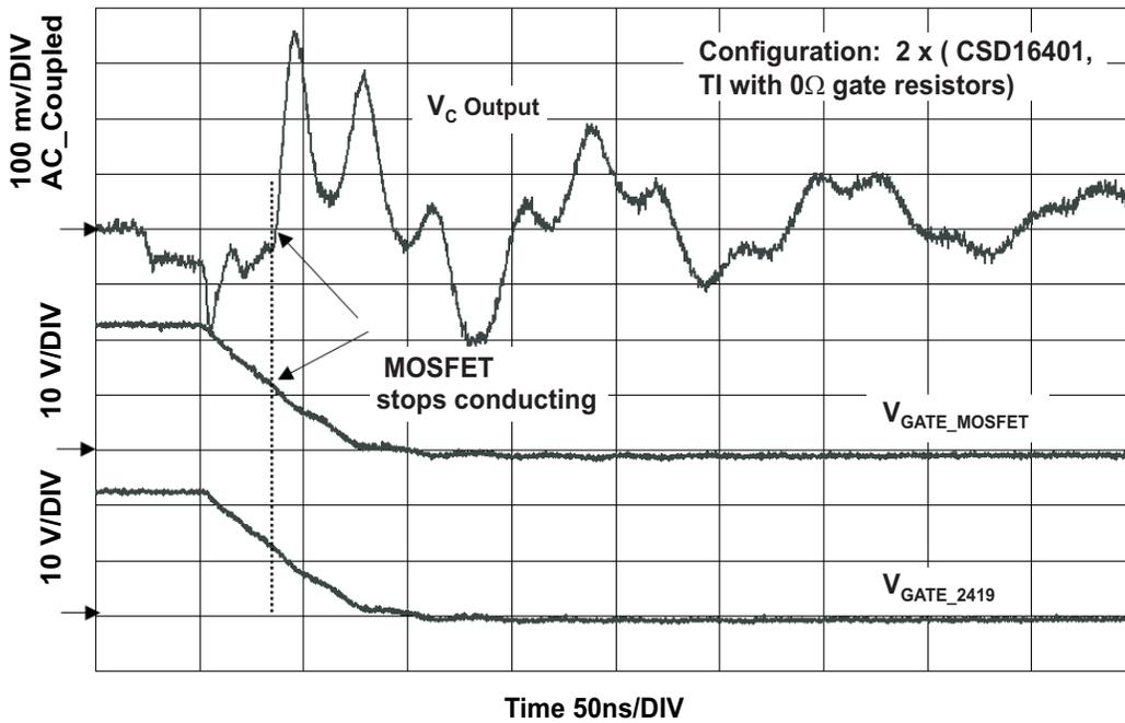
Figure 14. Gate Turnoff Waveforms with R<sub>GATE</sub> = 0Ω
