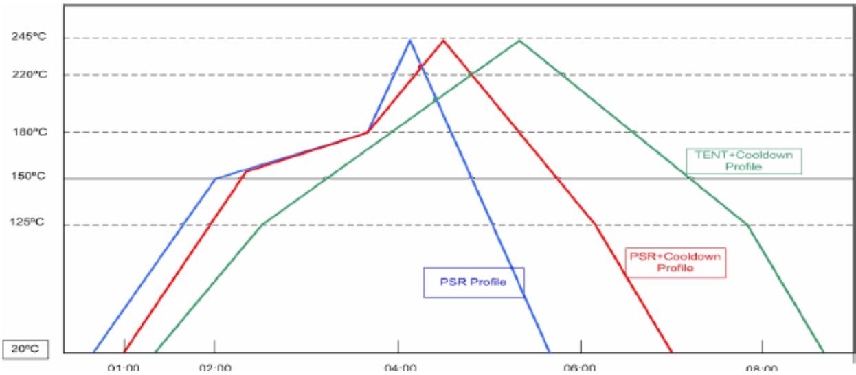
Figure 5-5: Reflow Temperature Profile.
