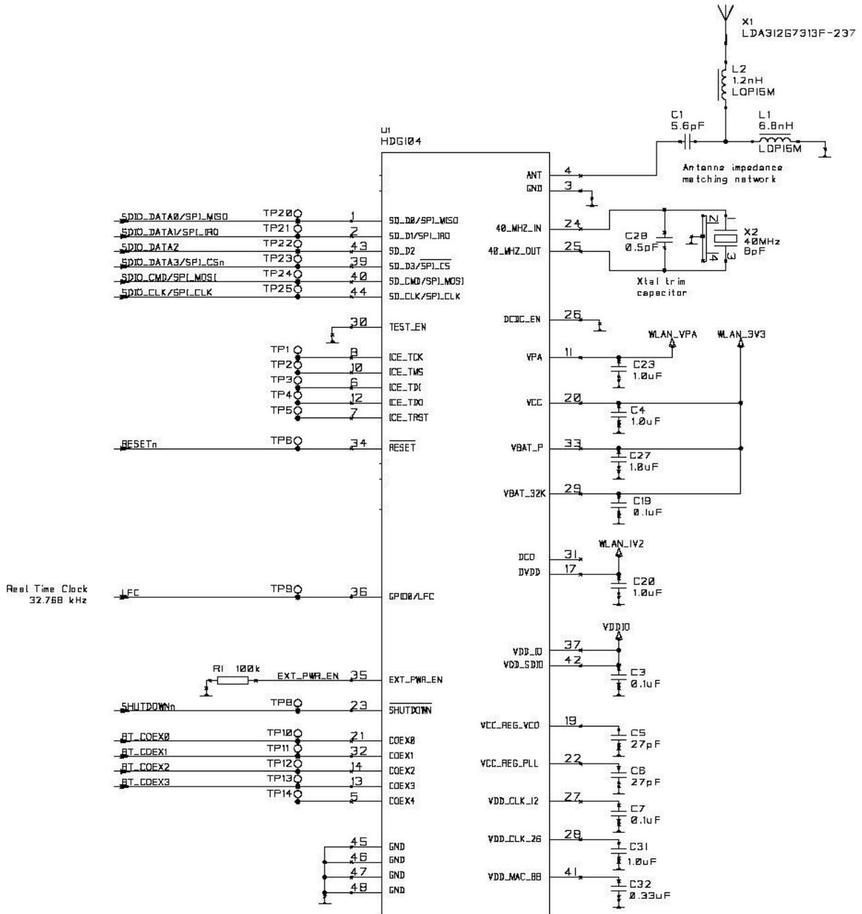
Figure 5-6: Reference design schematic.
