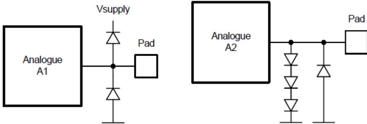
Figure 3-5: Schematics of analogue inputs A1 and A2
