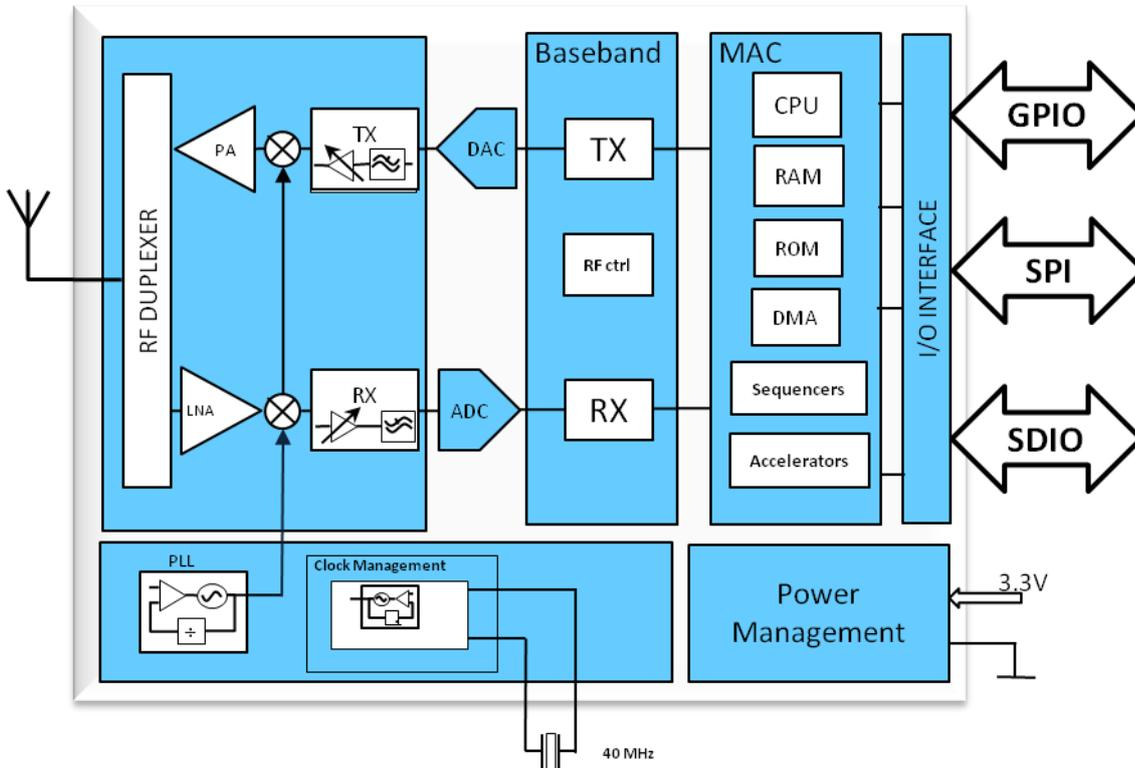
Figure 2.1: Block diagram.
