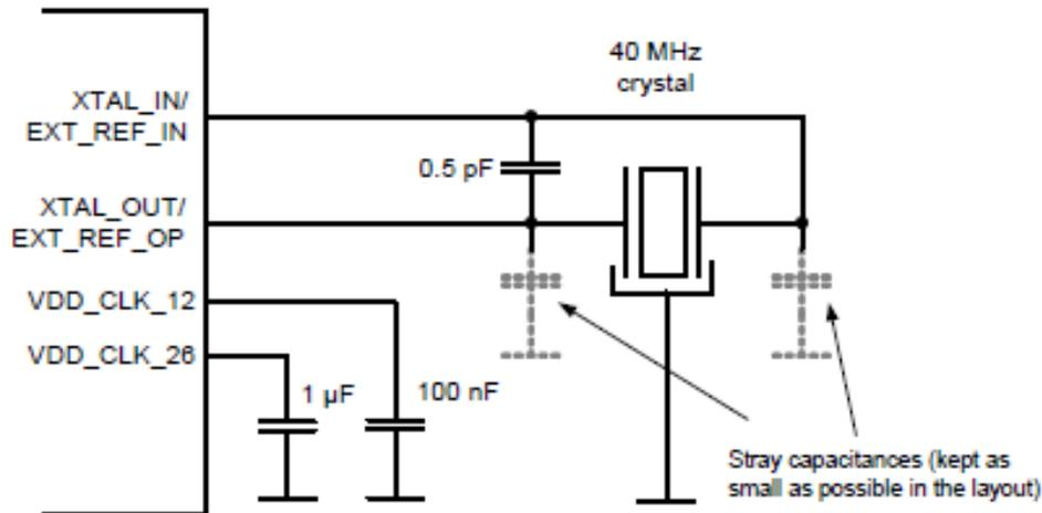
Figure 5-1: Reference clock setup
