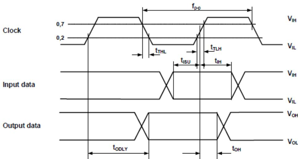
Figure 3-2: SDIO timing diagram (high speed mode)
