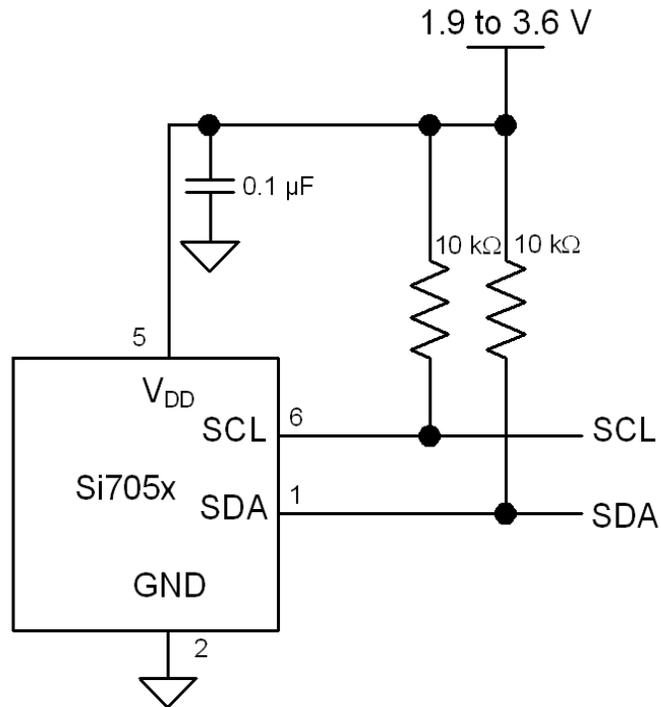
**Figure 2. Typical Application Circuit for Temperature Measurement**
