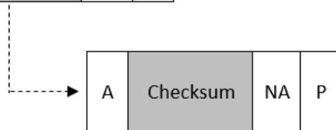
**\*Note:** Device will NACK the slave address byte until conversion is complete.
