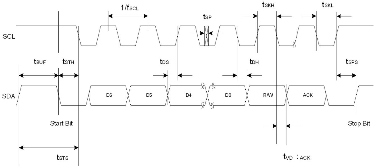
Figure 1. I<sup>2</sup>C Interface Timing Diagram
