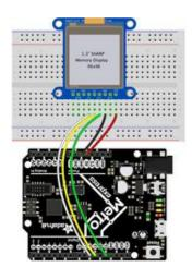
Microcontroller GND to LCD Gnd Microcontroller 5V to LCD Vin Microcontroller D13 to LCD Clk Microcontroller D11 to LCD DI Microcontroller D10 to LCD CS
