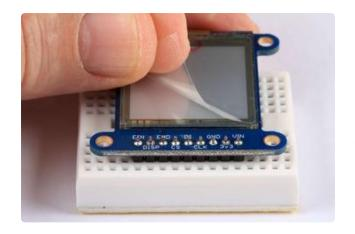
Remove the Protective Film After soldering is complete. Gently peel the film from the display.
