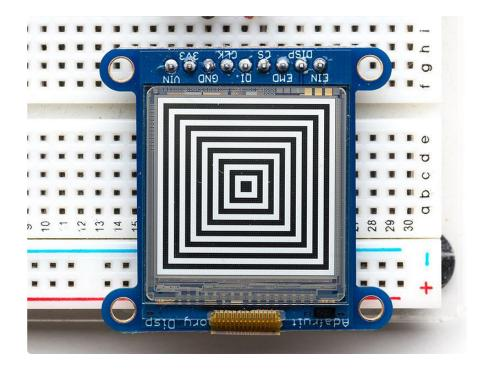
The 1.3" SHARP Memory LCD display is a cross between an elnk (e-paper) display and an LCD. It has the ultra-low power usage of elnk and the fast-refresh rates of an LCD. This model has a matt silver background, and pixels show up as little mirrors for a silver-reflective display, a really beautiful and unique look. It does not have a backlight, but it is daylight readable. For dark/night reading you may need to illuminate the LCD area with external LEDs.
