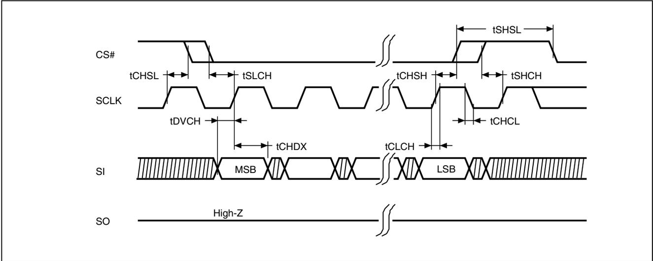
**Figure 47. Output Timing**
