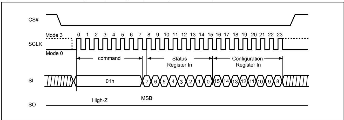
The CS# must go high exactly at the byte boundary; otherwise, the instruction will be rejected and not executed. The self-timed Write Status Register cycle time (tW) is initiated as soon as Chip Select (CS#) goes high. The Write in Progress (WIP) bit still can be checked out during the Write Status Register cycle is in progress. The WIP sets 1 during the tW timing, and sets 0 when Write Status Register Cycle is completed, and the Write Enable Latch (WEL) bit is reset.
