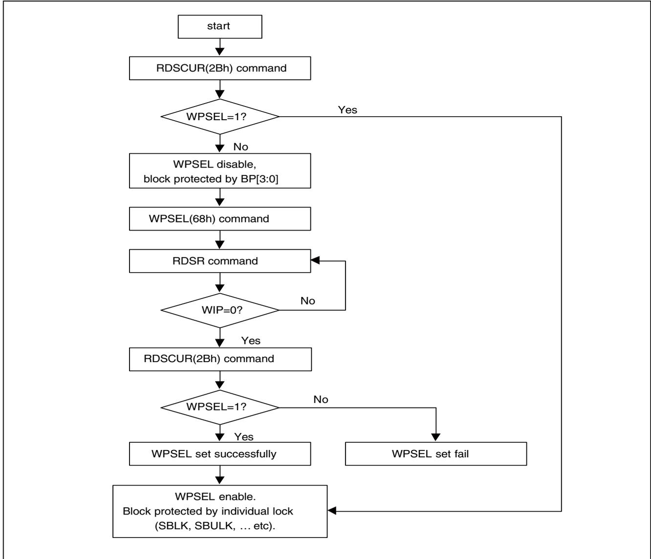
**9-30. Single Block Lock/Unlock Protection (SBLK/SBULK)**
