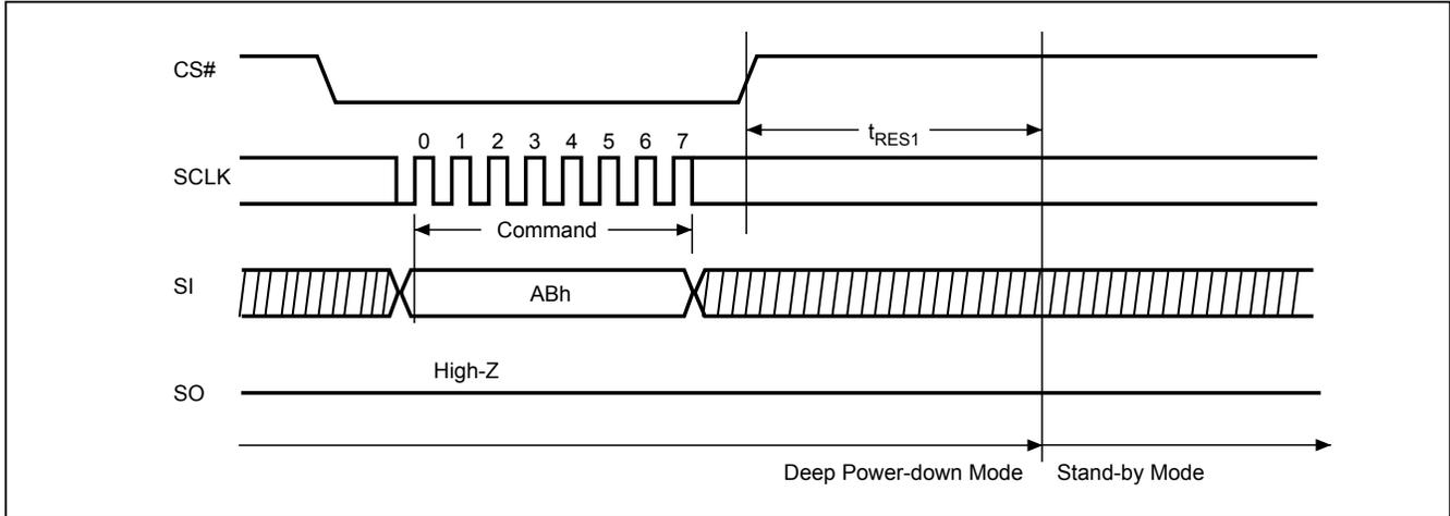
**9-23. Read Electronic Manufacturer ID & Device ID (REMS), (REMS2), (REMS4)**
