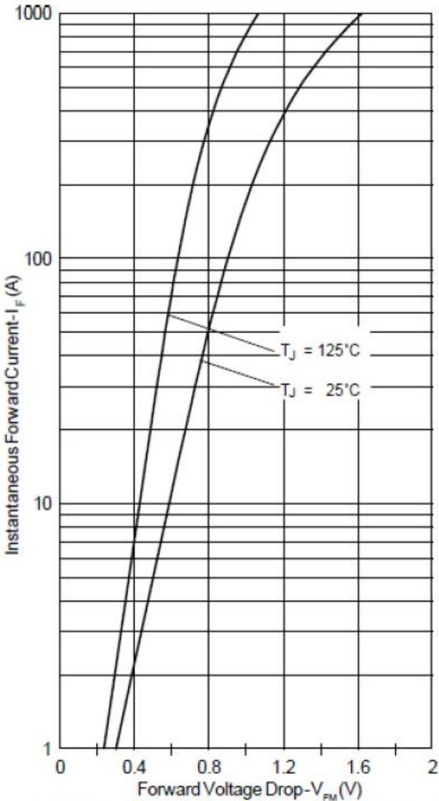
Fig. 1 - Max. Forward Voltage Drop Characteristics
