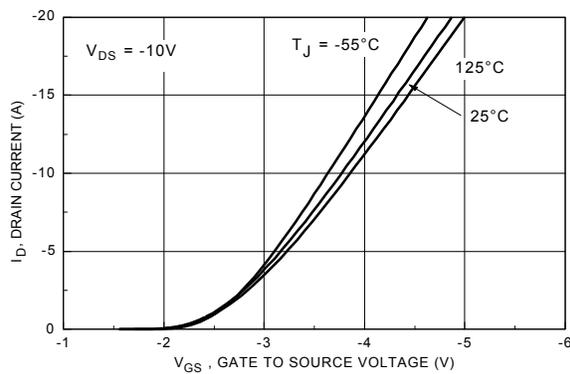
Figure 5. Transfer Characteristics.
