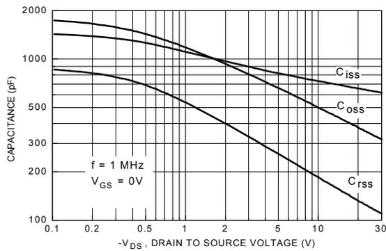
Figure 9. Capacitance Characteristics.
