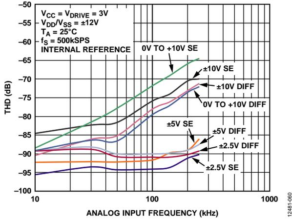
Figure 10. THD vs. Analog Input Frequency for Single-Ended (SE) and True Differential (Diff) Mode at 3 V<sub>CC</sub>
