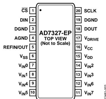
Figure 3. Pin Configuration
