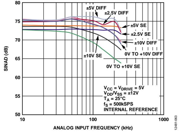
Figure 13. SINAD vs. Analog Input Frequency for Single-Ended (SE) and True Differential (Diff) Mode at 5 V<sub>CC</sub>
