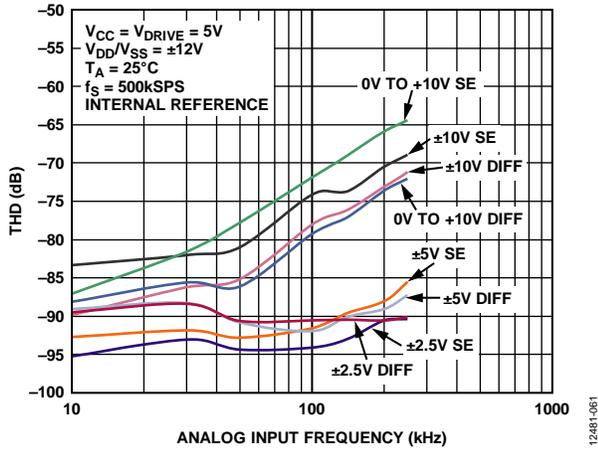
Figure 11. THD vs. Analog Input Frequency for Single-Ended (SE) and True Differential (Diff) Mode at 5 V<sub>CC</sub>
