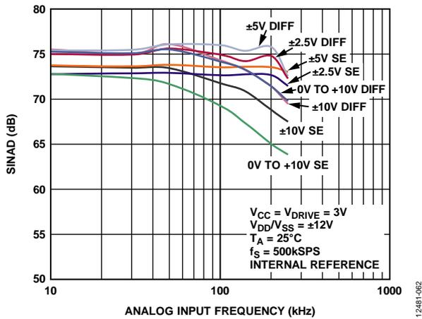
Figure 12. SINAD vs. Analog Input Frequency for Single-Ended (SE) and True Differential (Diff) Mode at 3 V<sub>CC</sub>
