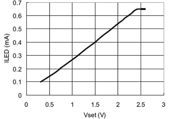
**Typical Performance Characteristics** (continued) (@ $T_A = +25^\circ\text{C}$ ,  $C_{IN} = 10\mu\text{F}$ ,  $C_O = 10\mu\text{F}$ ,  $L = 4.7\mu\text{H}$ , unless otherwise specified.)
