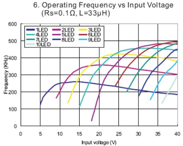
**Typical Performance Characteristics** (continued) (@T<sub>A</sub> = +25°C, V<sub>IN</sub> = 16V, unless otherwise specified.)
