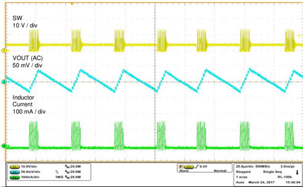
$V_{IN} = 3.6\text{ V}, V_{OUT} = 12\text{ V}, I_{OUT} = 3\text{ mA}$
