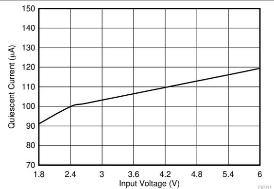
Figure 6-6. Quiescent Current into VIN vs Input Voltage
