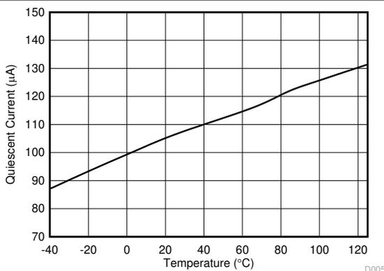
Figure 6-5. Quiescent Current into VIN vs Temperature
