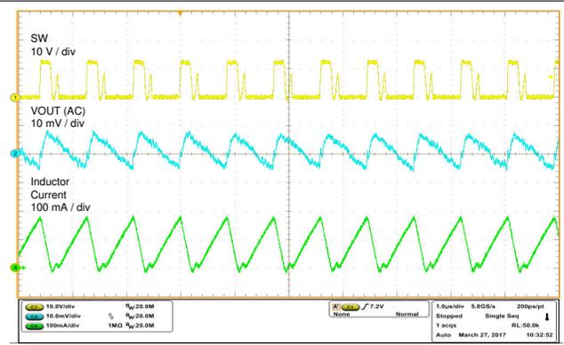
$V_{IN} = 3.6\text{ V}, V_{OUT} = 12\text{ V}, I_{OUT} = 18\text{ mA}$
