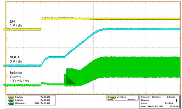
$V_{IN} = 3.6\text{ V}, V_{OUT} = 12\text{ V}, I_{OUT} = 50\text{ mA}$
