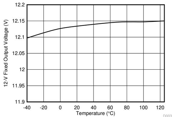
Figure 6-3. 12-V Fixed Output Voltage vs Temperature
