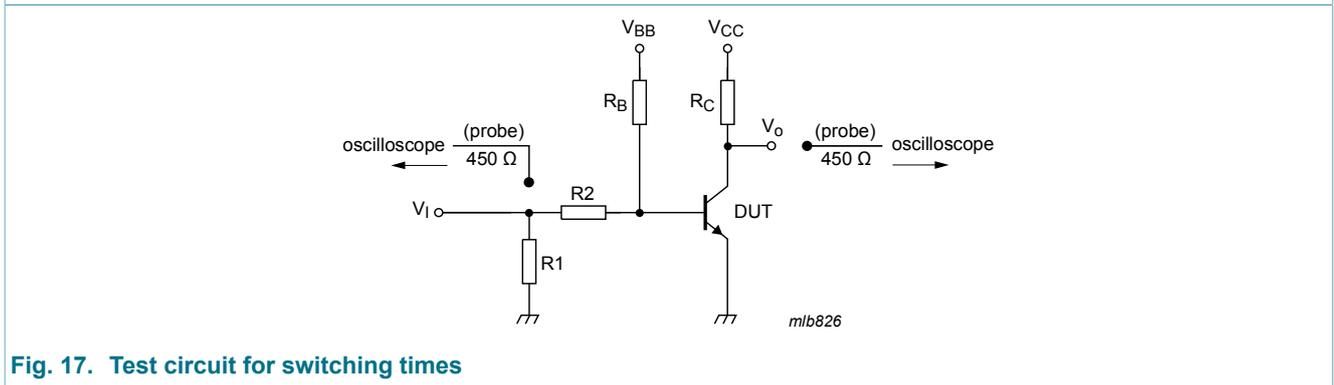
Fig. 17. Test circuit for switching times
