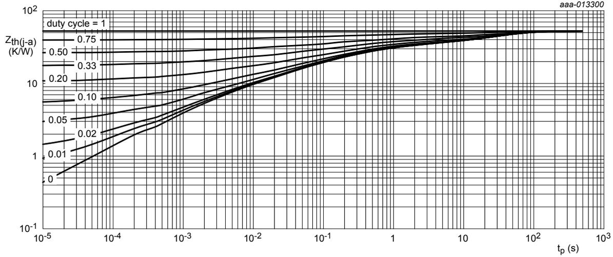
FR4 PCB, 4-layer copper, mounting pad for collector  $1 \text{ cm}^2$
