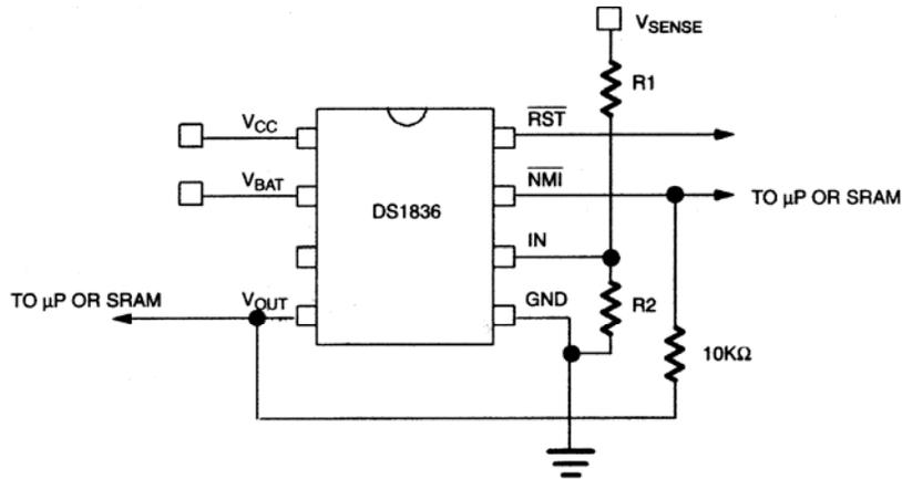
$$V_{\text{SENSE}} = \frac{R1 + R2}{R2} \times 1.25$$
