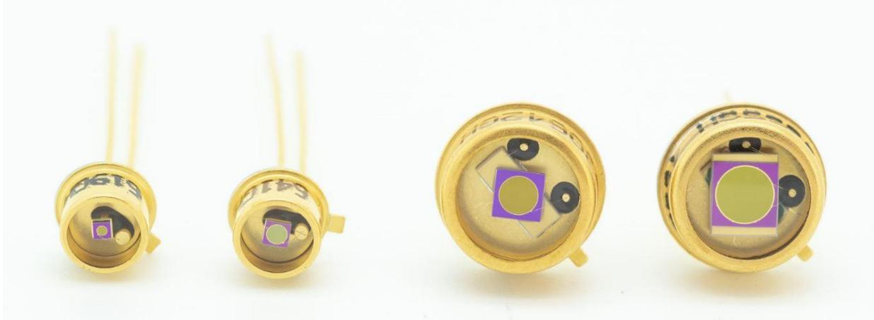
Excelitas' Large Area PIN Diodes are highly sensitive, low capacitance InGaAs diodes that provide high responsivity from 800 nm to 1700 nm. An ultra-low capacitance version for high bandwidth applications is available upon request.
