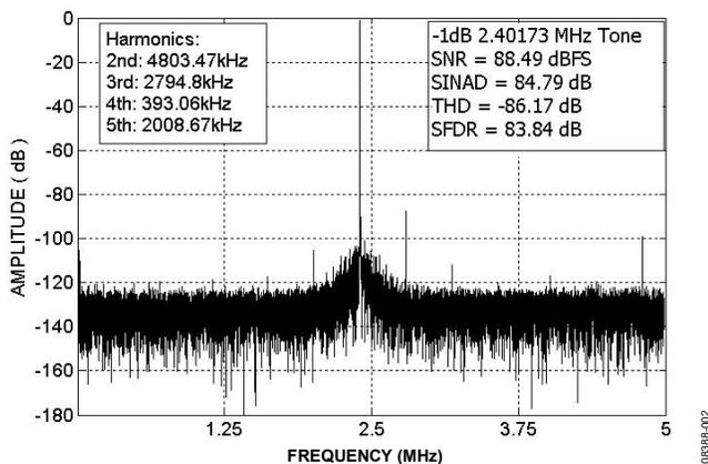
Figure 2. AD7626 Output, 64,000 Point, FFT Plot,  $-1$  dBFS Amplitude, 2.40173 MHz Input Tone, 10.000 MSPS Sampling Rate
