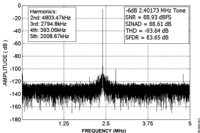
Figure 3. AD7626 Output, 64,000-Point FFT Plot,  $-6$  dBFS Amplitude, 2.40173 MHz Input Tone, 10.000 MSPS Sampling Rate
