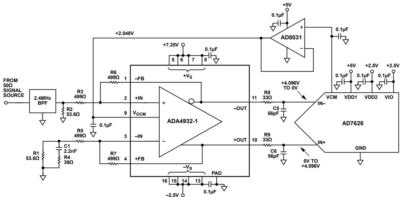
Figure 1 . ADA4932-1 Driving the AD7626 (All Connections and Decoupling Not Shown)
