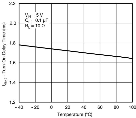
**Fig. 18 - Turn-On Delay Time vs. Temperature**
