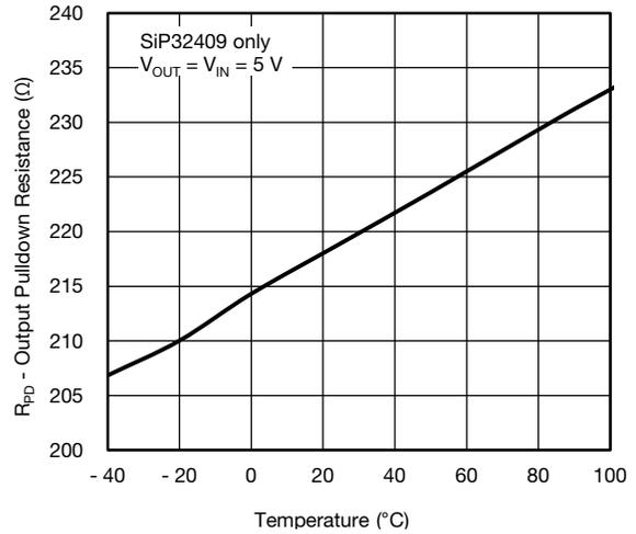
Fig. 15 - Output Pull-down Resistance vs. Temperature
