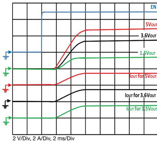
**Fig. 23 - Typical Turn-on Delay, Rise Time**
