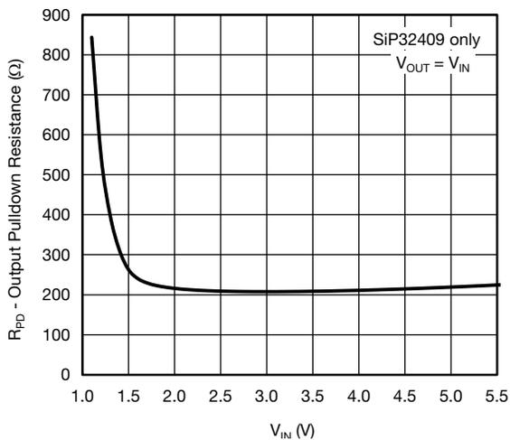
Fig. 13 - Output Pull-down Resistance vs. Input Voltage
