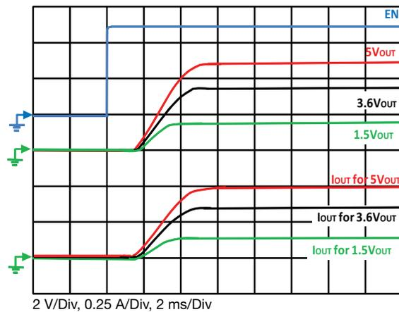
**Fig. 22 - Typical Turn-on Delay, Rise Time**
