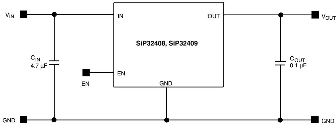
Fig. 1 - SiP32408, SiP32409 Typical Application Circuit
