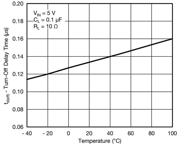
**Fig. 19 - Turn-Off Delay Time vs. Temperature**
