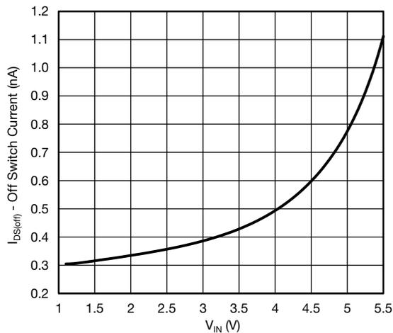
Fig. 8 - Off Switch Current vs. Input Voltage
