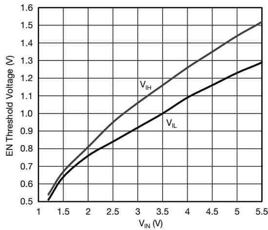
**Fig. 20 - EN Threshold Voltage vs. Input Voltage**
