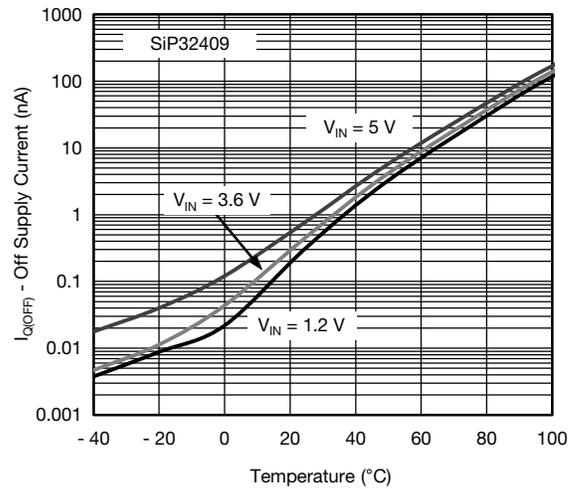
Fig. 10 - Off Supply Current vs. Temperature
