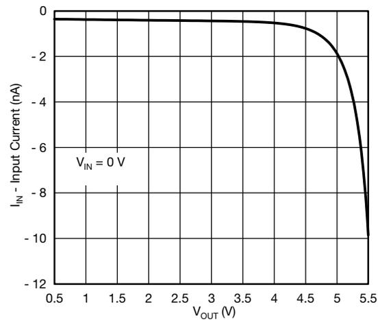
Fig. 16 - Reverse Blocking Current vs. Output Voltage
