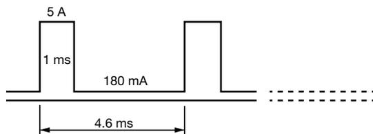
SiP32408 and SiP32409 can safely support 5 A pulse current repetitively at 25 °C.
