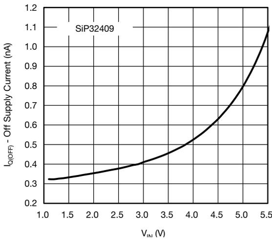
Fig. 7 - Off Supply Current vs. Input Voltage
