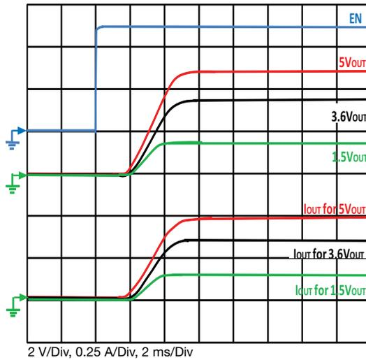
**Fig. 27 - Typical Turn-on Delay, Rise Time**
