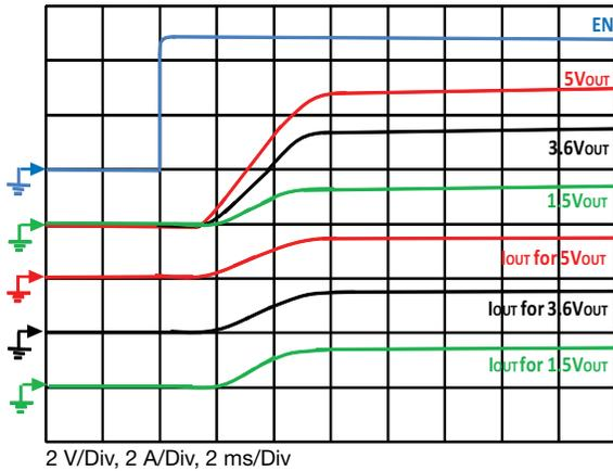
**Fig. 21 - Typical Turn-on Delay, Rise Time**
