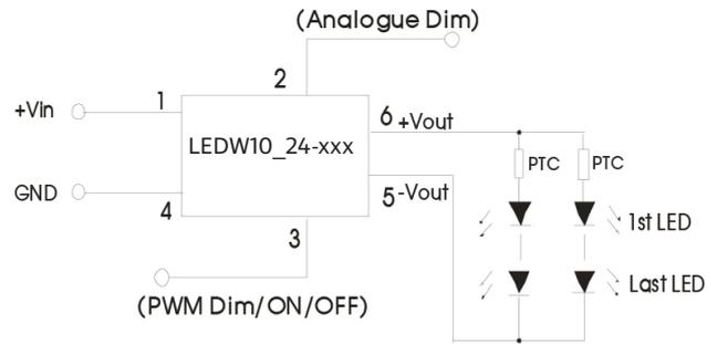
If it is necessary to protect LED in actual application, you could connect a PTC to the input of every channel or all channels, as shown in Recommended AC input circuit.
