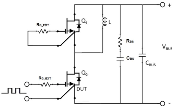
Figure 23. Schematic of the half-bridge mode switching test circuit. Note, a bus RC snubber ( $R_{BS} = 2.5\Omega$ ,  $C_{BS} = 100\text{nF}$ ) is used to reduce the power loop high frequency oscillations.
