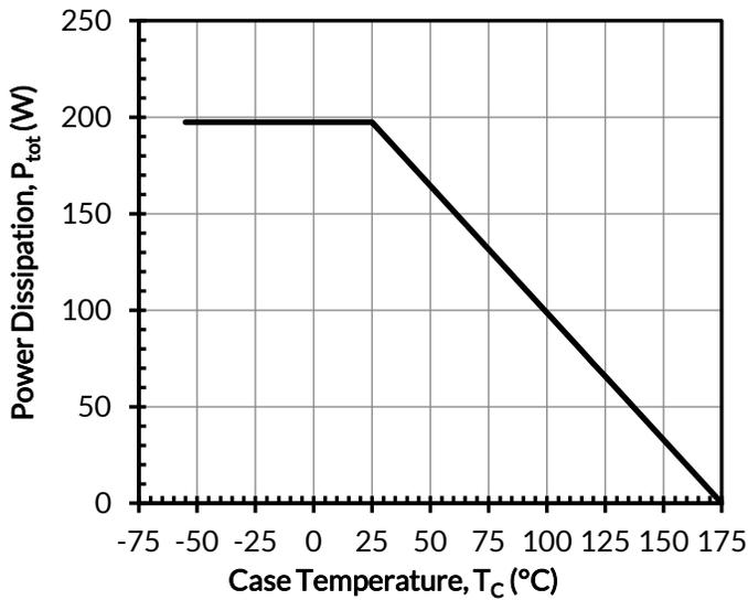
Figure 15. Total power dissipation
