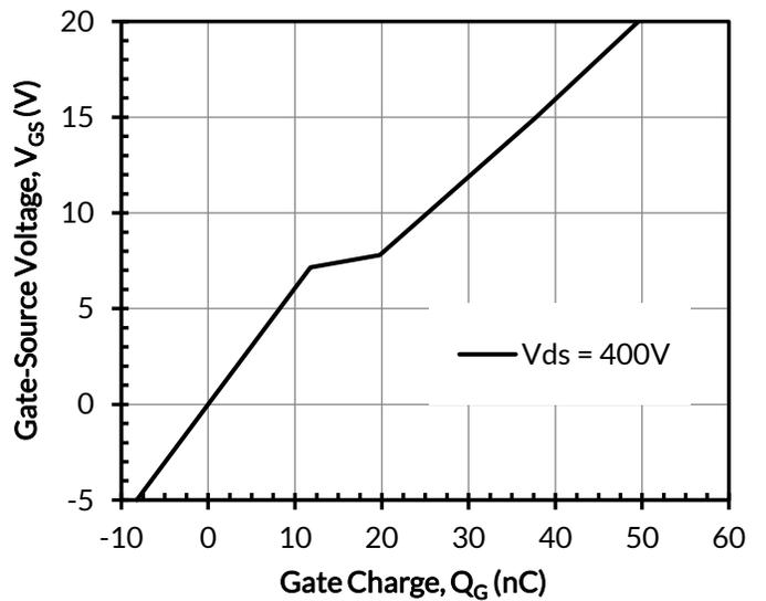
Figure 8. Typical gate charge at  $I_D = 30A$
