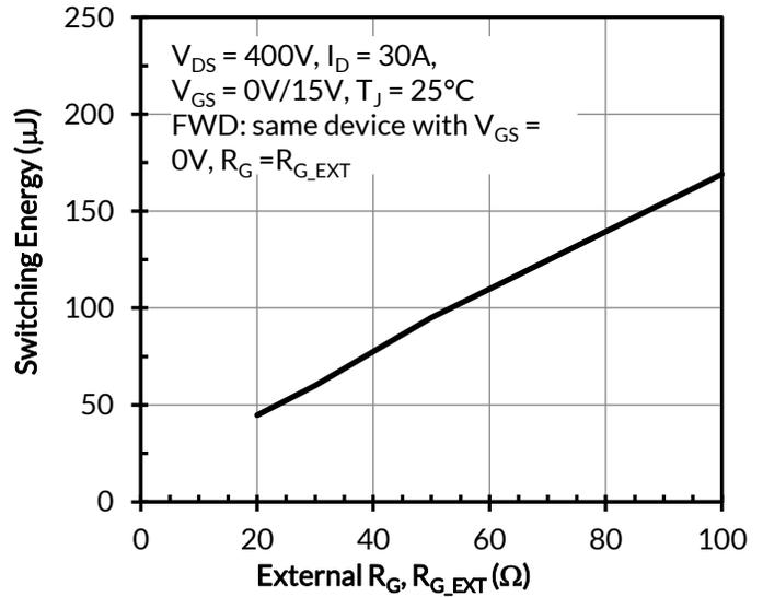
Figure 22. Clamped inductive switching turn-off energy vs.  $R_{G,EXT\_OFF}$
