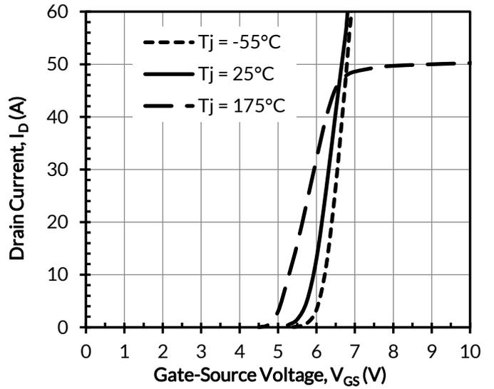
Figure 6. Typical transfer characteristics at  $V_{DS} = 5V$
