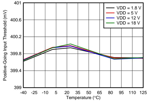
Figure 3. Rising Input Threshold Voltage ( $V_{IT+}$ ) vs Temperature
