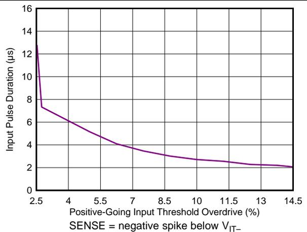
Figure 7. Minimum Pulse Width vs Threshold Overdrive Voltage
