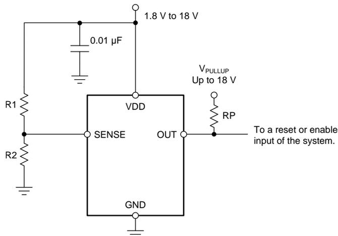
**Figure 15. Monitoring the Same Voltage as  $V_{DD}$**
