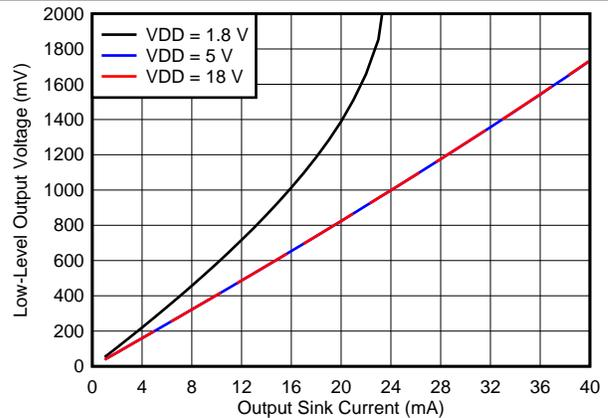
Figure 13. Output Voltage Low ( $V_{OL}$ ) vs Output Sink Current ( $125^\circ\text{C}$ )
