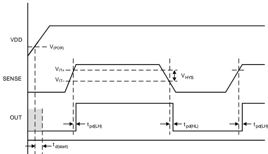
Figure 1. Timing Diagram
