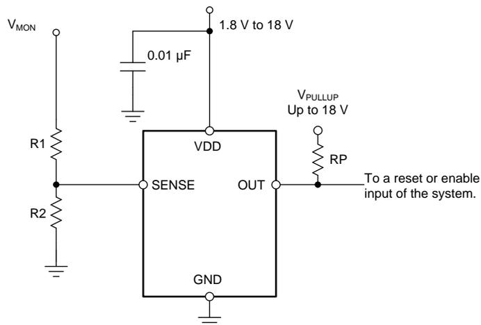
Figure 14. Interfacing to a Voltage Other Than  $V_{DD}$
