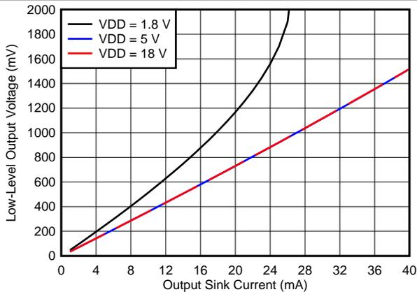
Figure 12. Output Voltage Low ( $V_{OL}$ ) vs Output Sink Current ( $85^\circ\text{C}$ )
