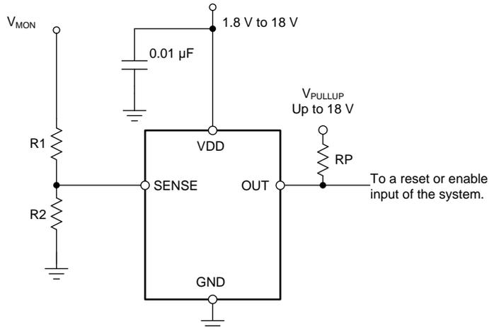
NOTE: The input can monitor a voltage greater than maximum  $V_{DD}$  with the use of an external resistor divider network.
