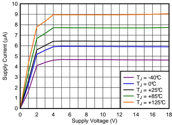
Figure 2. Supply Current ( $I_{DD}$ ) vs Supply Voltage ( $V_{DD}$ )
