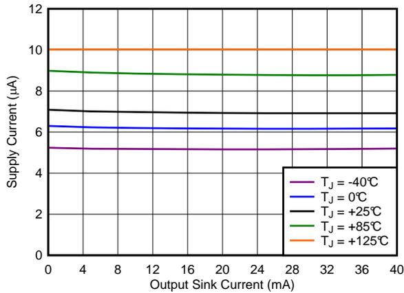
Figure 8. Supply Current ( $I_{DD}$ ) vs Output Sink Current
