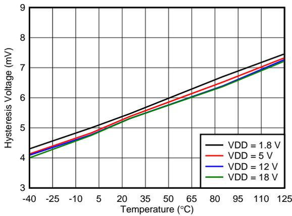
Figure 4. Hysteresis ( $V_{hys}$ ) vs Temperature
