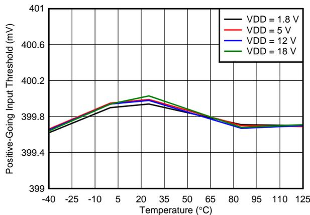
**Figure 18. Rising Input Threshold Voltage ( $V_{IT+}$ ) vs Temperature**
