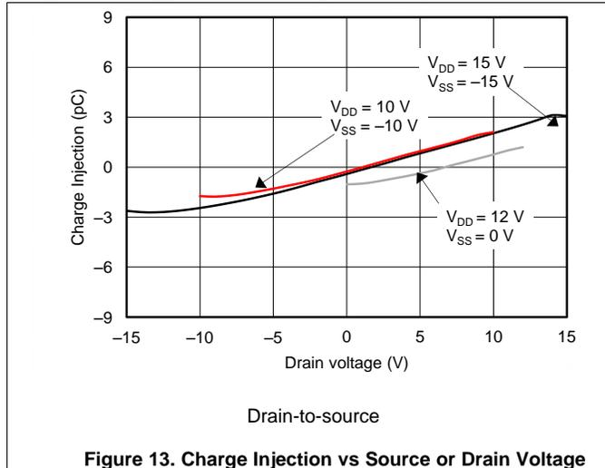
Figure 13. Charge Injection vs Source or Drain Voltage
