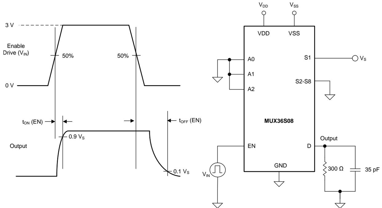
Figure 32. Turn-On and Turn-Off Time Measurement Setup
