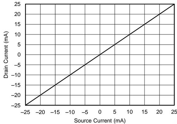
Figure 25. Source Current vs Drain Current
