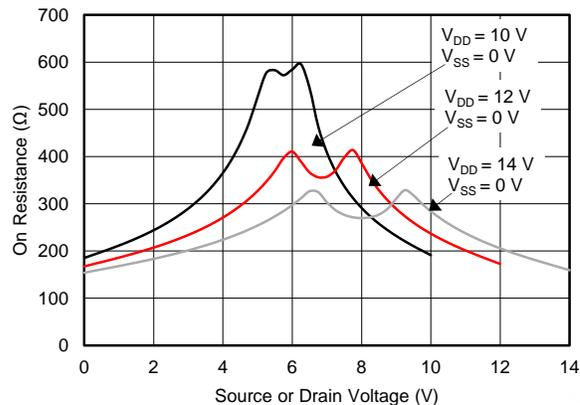
Figure 6. On-Resistance vs Source or Drain Voltage
