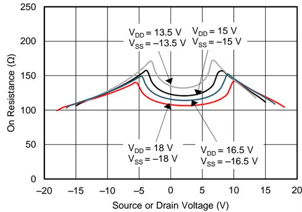
**Figure 45. On-Resistance Variation With Supply and Input Voltage**
