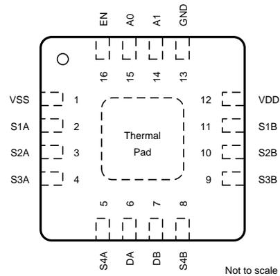
RUM and RRJ have the same package dimension, but different thermal pad dimension and lead finger length.
