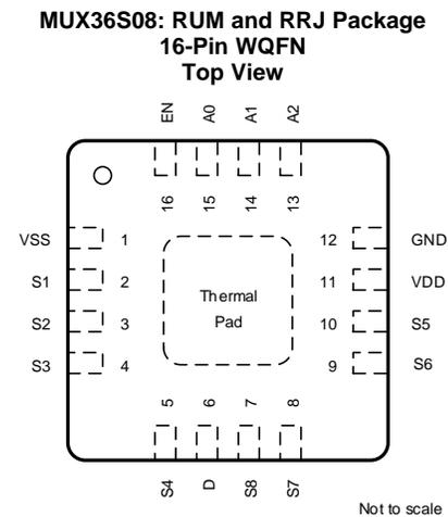
RUM and RRJ have the same package dimension, but different thermal pad dimension and lead finger length.
