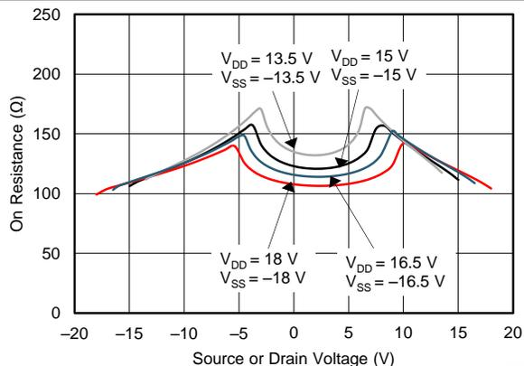
Figure 1. On-Resistance vs Source or Drain Voltage
