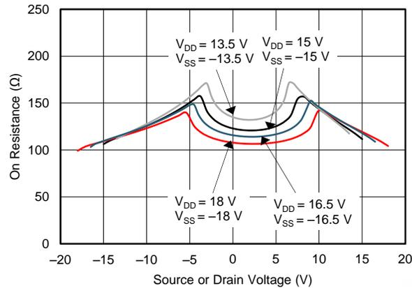
**Figure 42. On-Resistance vs Source or Drain Voltage**
