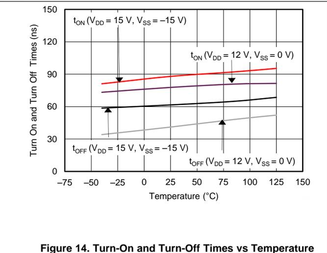
Figure 14. Turn-On and Turn-Off Times vs Temperature
