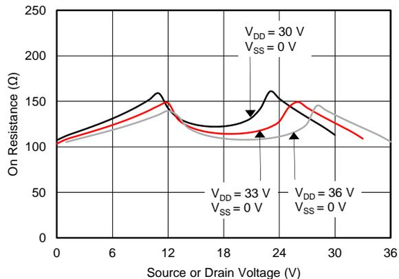
Figure 5. On-Resistance vs Source or Drain Voltage
