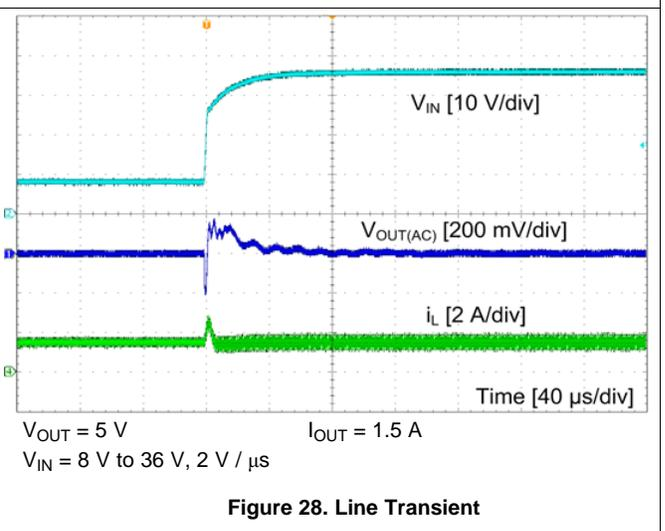
Unless otherwise specified the following conditions apply:  $V_{IN} = 12\text{ V}$ ,  $f_{SW} = 1600\text{ kHz}$ ,  $L = 4.7\text{ }\mu\text{H}$ ,  $C_{OUT} = 47\text{ }\mu\text{F}$ ,  $T_A = 25^\circ\text{C}$ .
