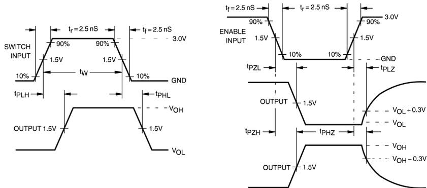
FIGURE 2. AC Waveforms
