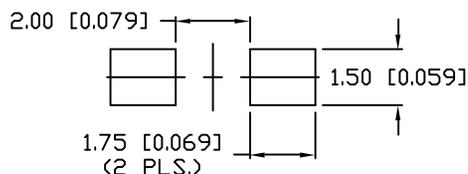
\*UNLESS OTHERWISE SPECIFIED TOLERANCES PER DECIMAL PRECISION ARE: X=±1 (±0.039), X.X=±0.5 (±0.020), X.XX=±0.25 (±0.010), X.XXX=±0.127 (±0.005). LEAD SIZE=±0.05 (0.002), LEAD LENGTH=±0.75 (±0.030). MIN.= +DECIMAL PRECISION -0.00, MAX.= +0.00 -DECIMAL PRECISION
