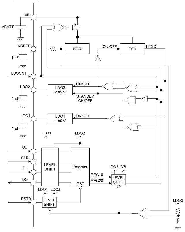
All the logic portions to which the power supply is not connected are connected to VB as power supplies.
